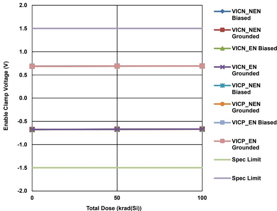
**Figure 3. HS-26C32EH enable input clamp voltage as a function of biased ([Figure 2](#)) and unbiased (grounded) LDR irradiation to 100krad(Si). The sample size for each of the LDR cells was 16. The SMD limits are -1.5V to 1.5V.**
