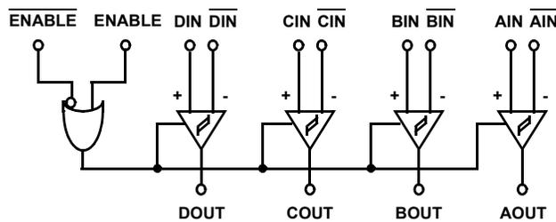
Figure 1. HS-26C32EH Block Diagram
