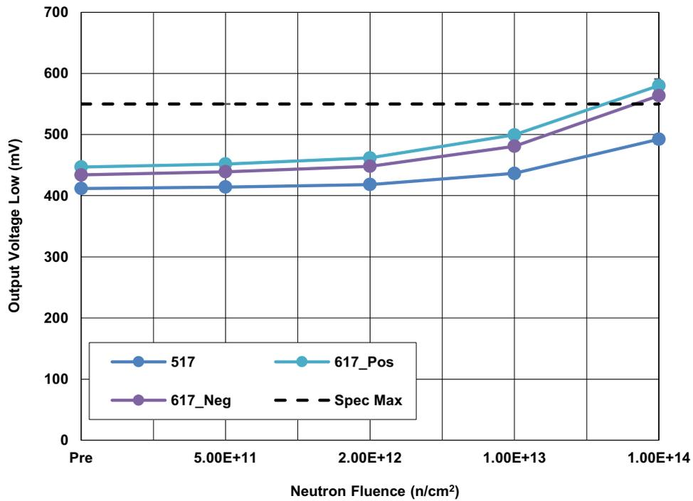
Figure 10. ISL70x17SEH low output voltage ( $V_{OL}$ ) at  $\pm 18V$  with  $I_{OUT} = 7.5mA$  following irradiation to each level. The error bars represent the minimum and maximum measured values. The SMD limit is 550mV maximum.
