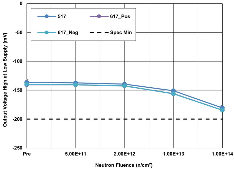
Figure 15. ISL70x17SEH high output voltage ( $V_{OH(LV)}$ ) with  $V_{CC} = 4V$ ,  $V_{EE} = -4V$ ,  $V_{CO} = 1.5V$ ,  $V_{EO} = -1.5V$ ,  $I_{OUT} = 1.5mA$  following irradiation to each level. The error bars represent the minimum and maximum measured values. The SMD limit is -200mV minimum.
