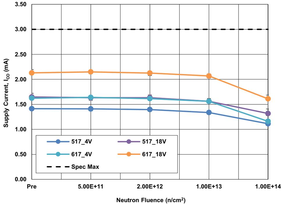
Figure 27. ISL70x17SEH supply current ( $I_{CO}$ ) at  $\pm 4V$  and  $\pm 18V$  following irradiation to each level. The error bars represent the minimum and maximum measured values. The SMD limit is 3mA maximum.
