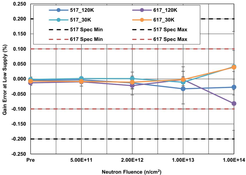
Figure 21. ISL70x17SEH gain error at low supply voltage ( $E_{GLV}$ ),  $V_{OUT} = \pm 0.1V$ ,  $R_{FB} = 120k$ , and  $30k$ ,  $G = 1$  following irradiation to each level. The error bars represent the minimum and maximum measured values. The SMD limits are  $-0.2\%$  minimum and  $0.2\%$  maximum for the ISL70517SEH and  $-0.1\%$  minimum and  $0.1\%$  maximum for the ISL70617SEH.
