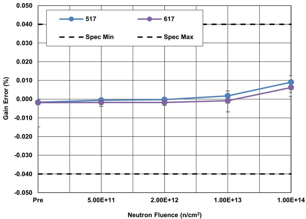
Figure 20. ISL70x17SEH gain error ( $E_G$ ) with  $V_{OUT} = \pm 2.5V$ ,  $RFB = 30k$ ,  $Gain = 1$  following irradiation to each level. The error bars represent the minimum and maximum measured values. The SMD limits are -0.04% minimum and 0.04% maximum.
