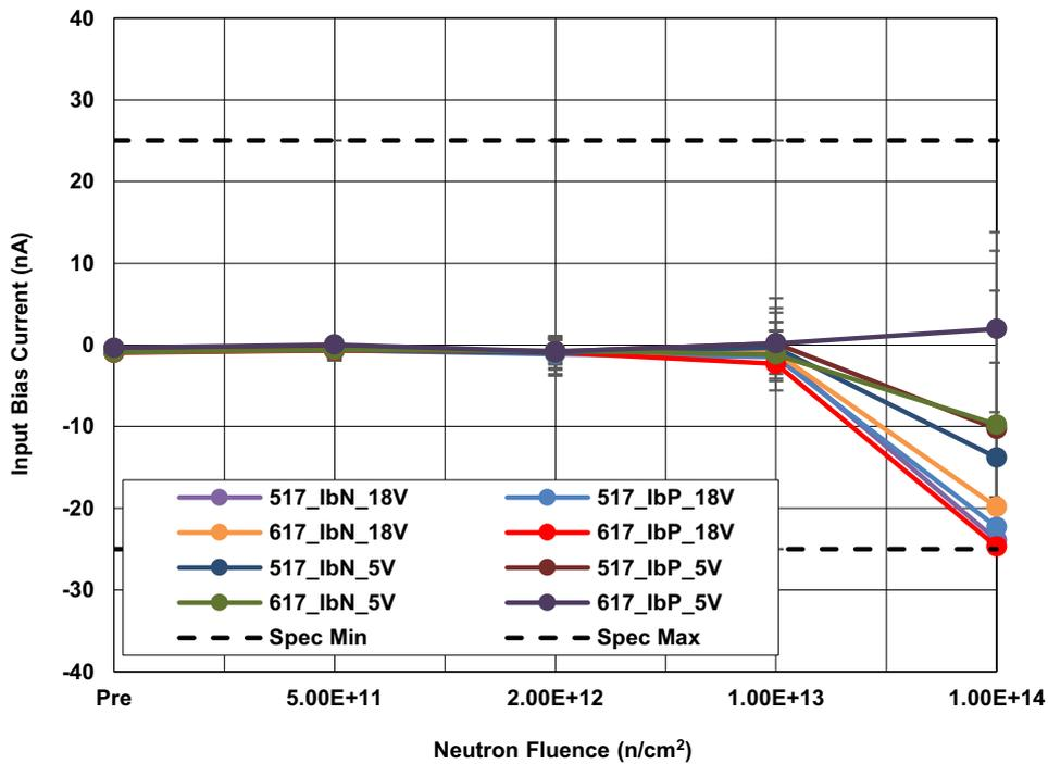
Figure 2. ISL70x17SEH input bias current ( $I_B$ ) at  $\pm 5V$  and  $\pm 18V$  following irradiation to each level. The error bars represent the minimum and maximum measured values. The SMD limits are  $-25nA$  minimum and  $25nA$  maximum.
