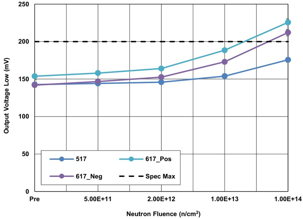
Figure 9. ISL70x17SEH low output voltage ( $V_{OL}$ ) at  $\pm 18V$  with  $I_{OUT} = 1.5mA$  following irradiation to each level. The error bars represent the minimum and maximum measured values. The SMD limit is 200mV maximum.
