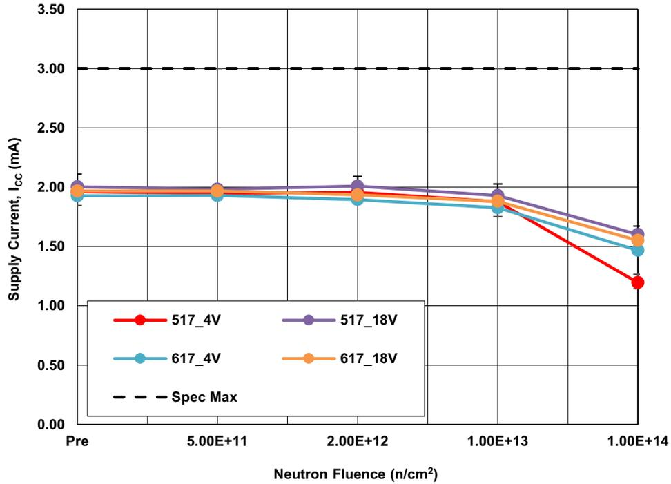
Figure 25. ISL70x17SEH supply current ( $I_{CC}$ ) at  $\pm 4V$  and  $\pm 18V$  following irradiation to each level. The error bars represent the minimum and maximum measured values. The SMD limit is 3mA maximum.
