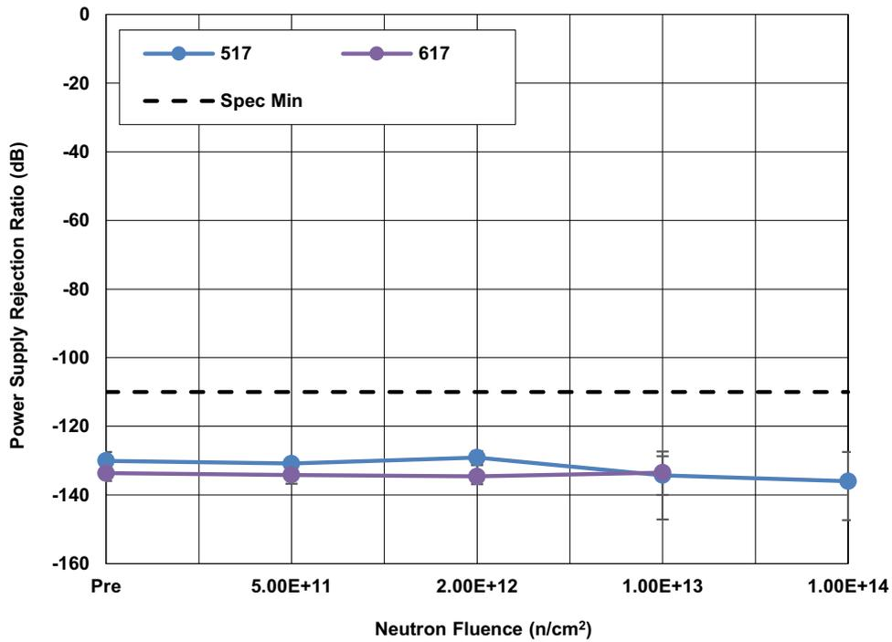
Figure 29. ISL70x17SEH input stage power supply rejection ratio (PSRRI) following irradiation to each level. The error bars represent the minimum and maximum measured values. The SMD limit is -110dB minimum.
