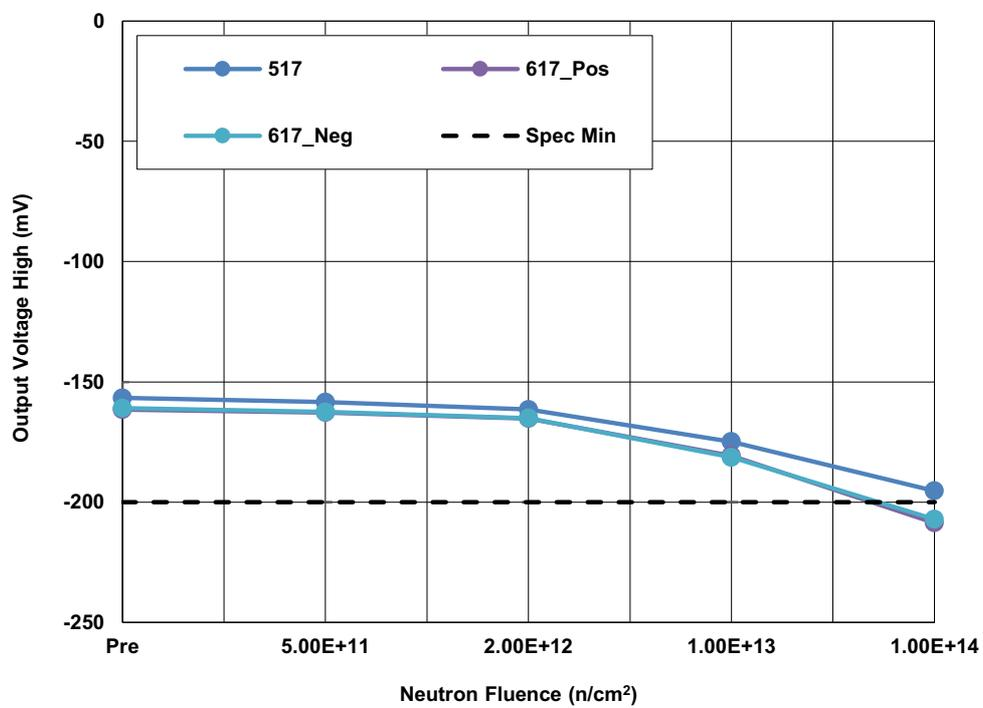
Figure 12. ISL70x17SEH high output voltage ( $V_{OH}$ ) at  $\pm 18V$  with  $I_{OUT} = -1.5mA$  following irradiation to each level. The error bars represent the minimum and maximum measured values. The SMD limit is -200mV maximum.
