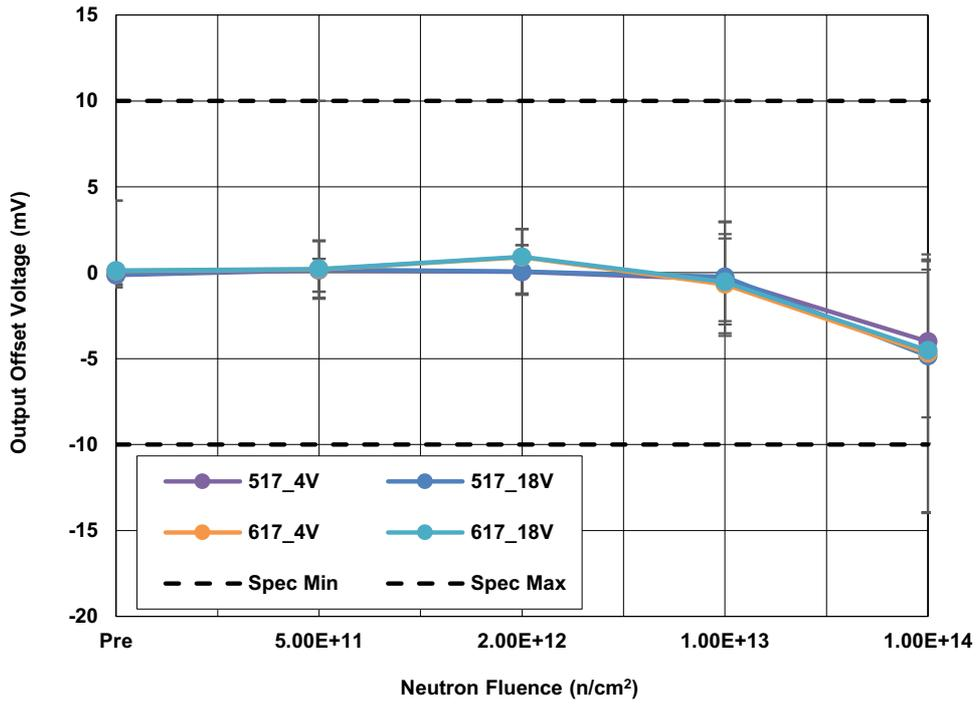
Figure 23. ISL70x17SEH output offset voltage ( $V_{OSOUT}$ ), at  $\pm 5V$  and  $\pm 18V$ , with  $R_{FB} = 30k$  following irradiation to each level. The error bars represent the minimum and maximum measured values. The SMD limits are  $-10mV$  minimum and  $10mV$  maximum.
