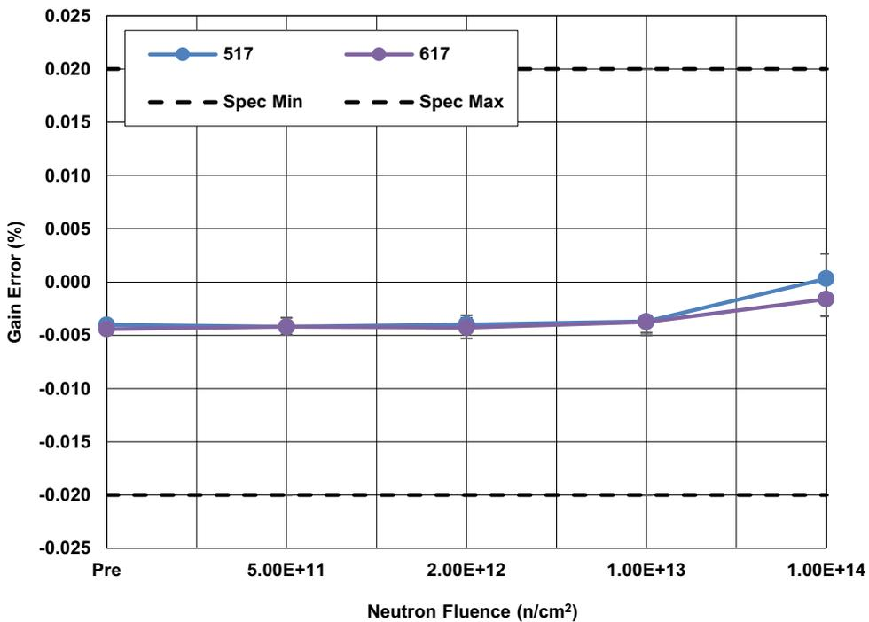
Figure 18. ISL70x17SEH gain error ( $E_G$ ) with  $V_{OUT} = \pm 10V$ ,  $R_{FB} = 120k$ ,  $Gain = 1$  following irradiation to each level. The error bars represent the minimum and maximum measured values. The SMD limits are -0.02% minimum and 0.02% maximum.
