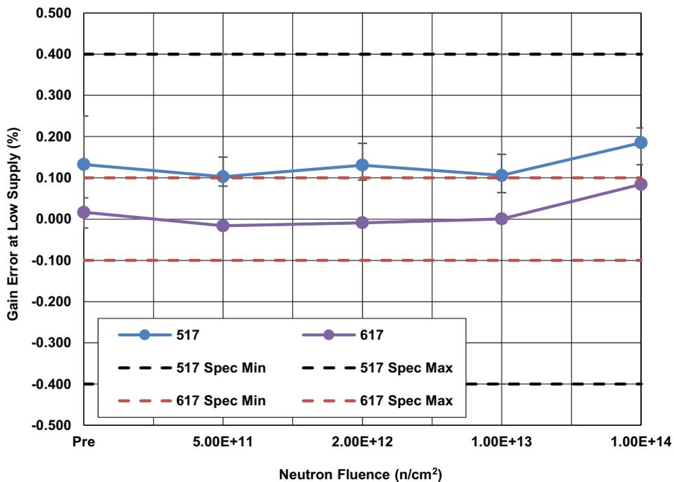
Figure 22. ISL70x17SEH gain error at low supply voltage ( $E_{GLV}$ ) with  $V_{OUT} = \pm 1.25V$ ,  $R_{FB} = 120k$ ,  $Gain = 100$  following irradiation to each level. The error bars represent the minimum and maximum measured values. The SMD limits are  $-0.4\%$  minimum and  $0.4\%$  maximum for the ISL70517SEH and  $-0.1\%$  minimum and  $0.1\%$  maximum for the ISL70617SEH.
