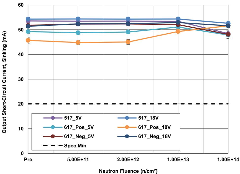
Figure 16. ISL70x17SEH output short-circuit current, sinking ( $I_{SC}$ ) at  $\pm 5V$  and  $\pm 18V$  following irradiation to each level. The error bars represent the minimum and maximum measured values. The SMD limit is 20mA minimum.
