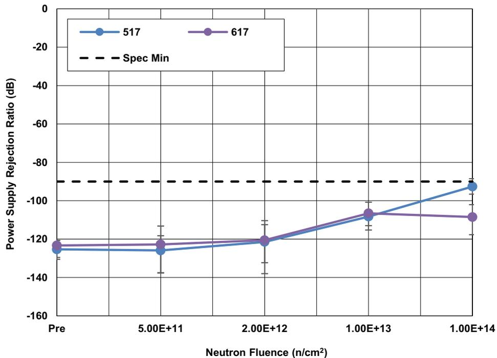
Figure 30. ISL70x17SEH output stage power supply rejection ratio (PSRRO) following irradiation to each level. The error bars represent the minimum and maximum measured values. The SMD limit is -90dB minimum.
