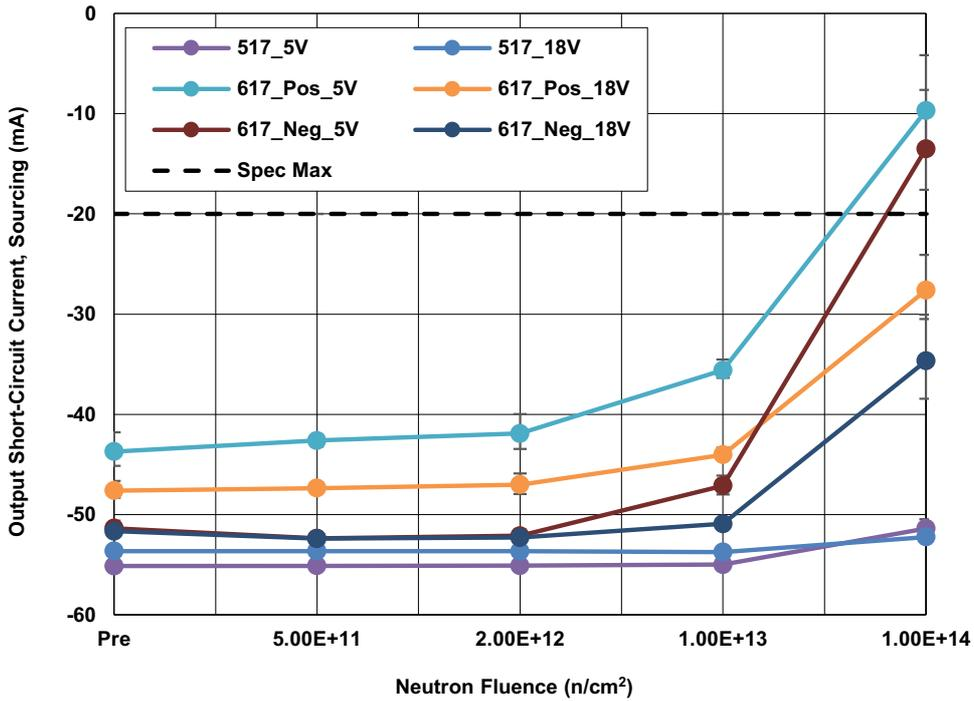
Figure 17. ISL70x17SEH output short-circuit current, sourcing ( $I_{SC}$ ) at  $\pm 5V$  and  $\pm 18V$  following irradiation to each level. The error bars represent the minimum and maximum measured values. The SMD limit is -20mA maximum.
