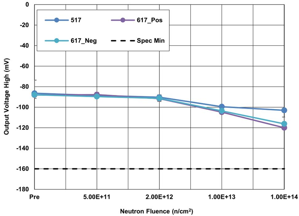
Figure 11. ISL70x17SEH high output voltage ( $V_{OH}$ ) at  $\pm 18V$  with  $I_{OUT} = 0mA$  following irradiation to each level. The error bars represent the minimum and maximum measured values. The SMD limit is -160mV minimum.
