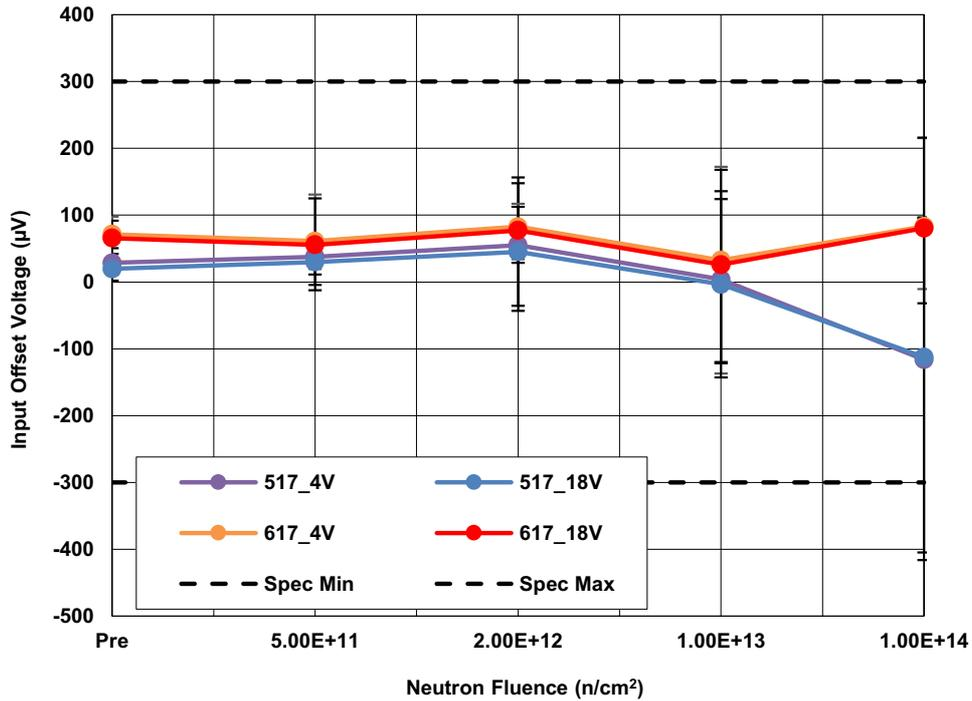
Figure 1. ISL70x17SEH input offset voltage ( $V_{OS}$ ) at  $\pm 4V$  and  $\pm 18V$  following irradiation to each level. The error bars represent the minimum and maximum measured values. The SMD limits are  $-300\mu V$  minimum and  $300\mu V$  maximum.
