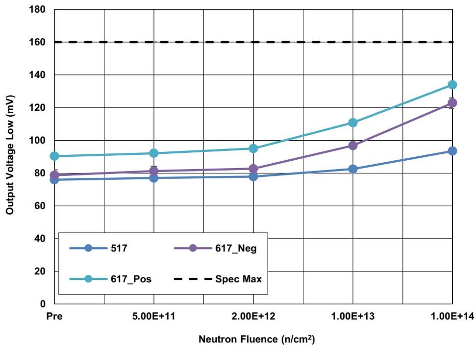
Figure 8. ISL70x17SEH low output voltage ( $V_{OL}$ ) at  $\pm 18V$  with  $I_{OUT} = 0mA$  following irradiation to each level. The error bars represent the minimum and maximum measured values. The SMD limit is 160mV maximum.
