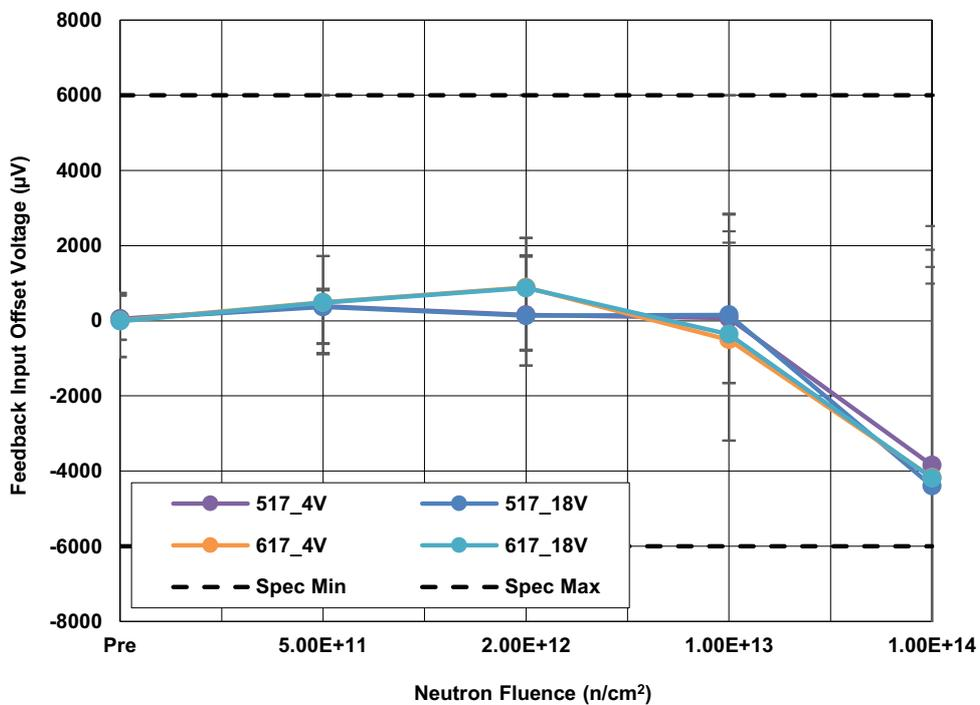
Figure 6. ISL70x17SEH feedback input offset voltage ( $V_{OSFB}$ ) at  $\pm 4V$  and  $\pm 18V$  following irradiation to each level. The error bars represent the minimum and maximum measured values. The SMD limit is -6000 $\mu V$  minimum and 6000 $\mu V$  maximum.
