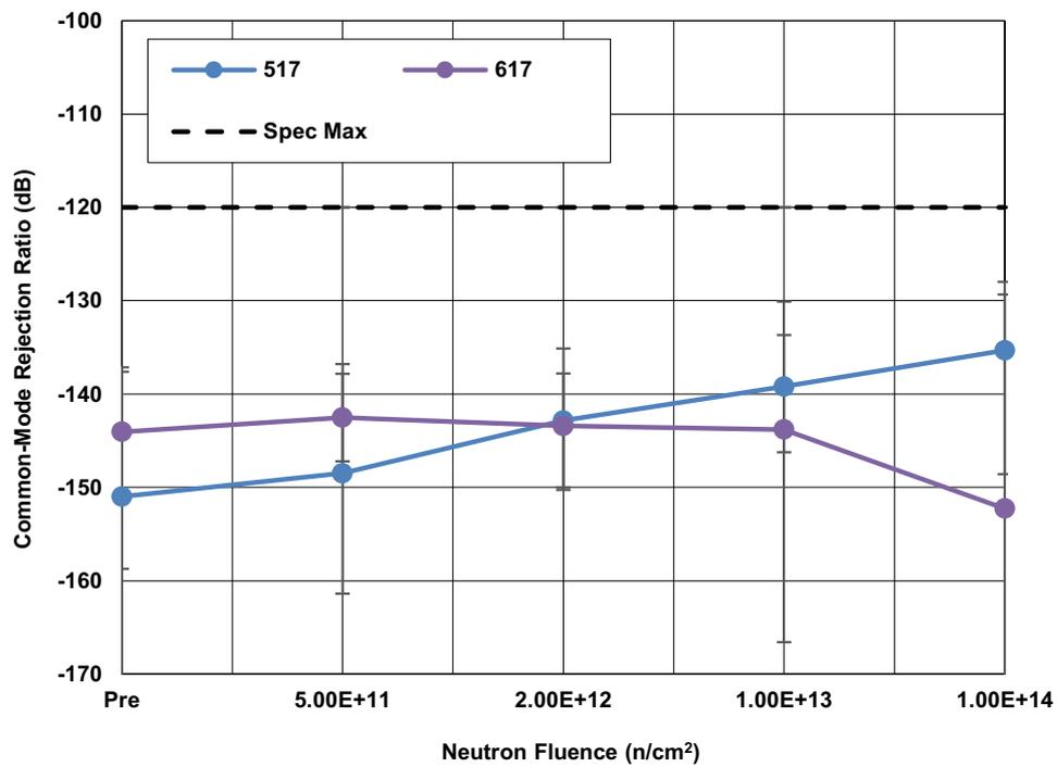
Figure 4. ISL70x17SEH common-mode rejection ratio (CMRR) with Gain = 100, following irradiation to each level. The error bars represent the minimum and maximum measured values. The SMD limit is  $-120dB$  maximum.
