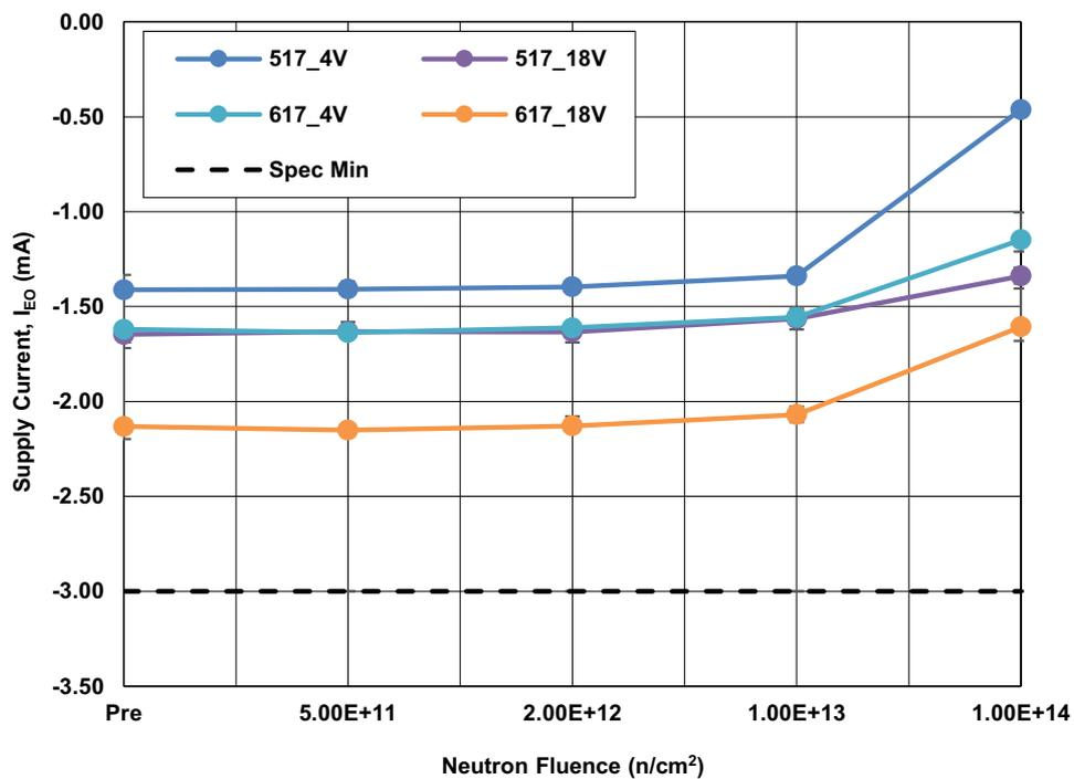
Figure 28. ISL70x17SEH supply current ( $I_{EO}$ ) at  $\pm 4V$  and  $\pm 18V$  following irradiation to each level. The error bars represent the minimum and maximum measured values. The SMD limit is -3mA minimum.
