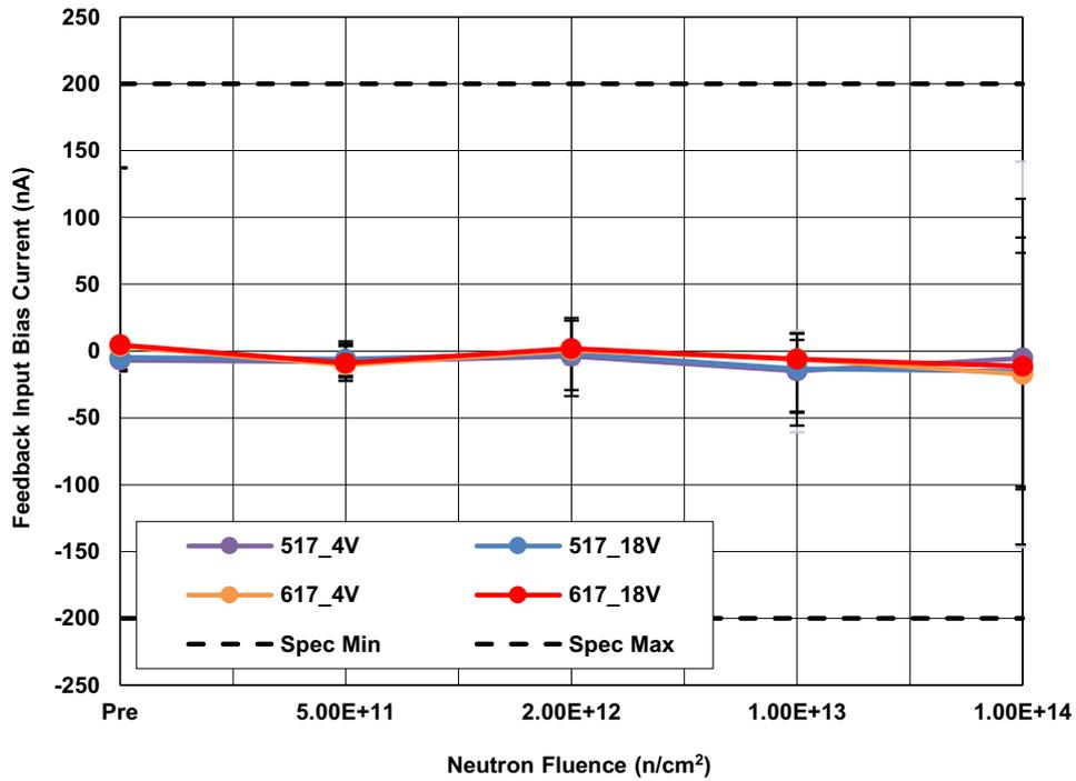
Figure 7. ISL70x17SEH feedback input bias current ( $I_{B_{FB}}$ ) at  $\pm 4V$  and  $\pm 18V$  following irradiation to each level. The error bars represent the minimum and maximum measured values. The SMD limit is -200nA minimum and 200nA maximum.
