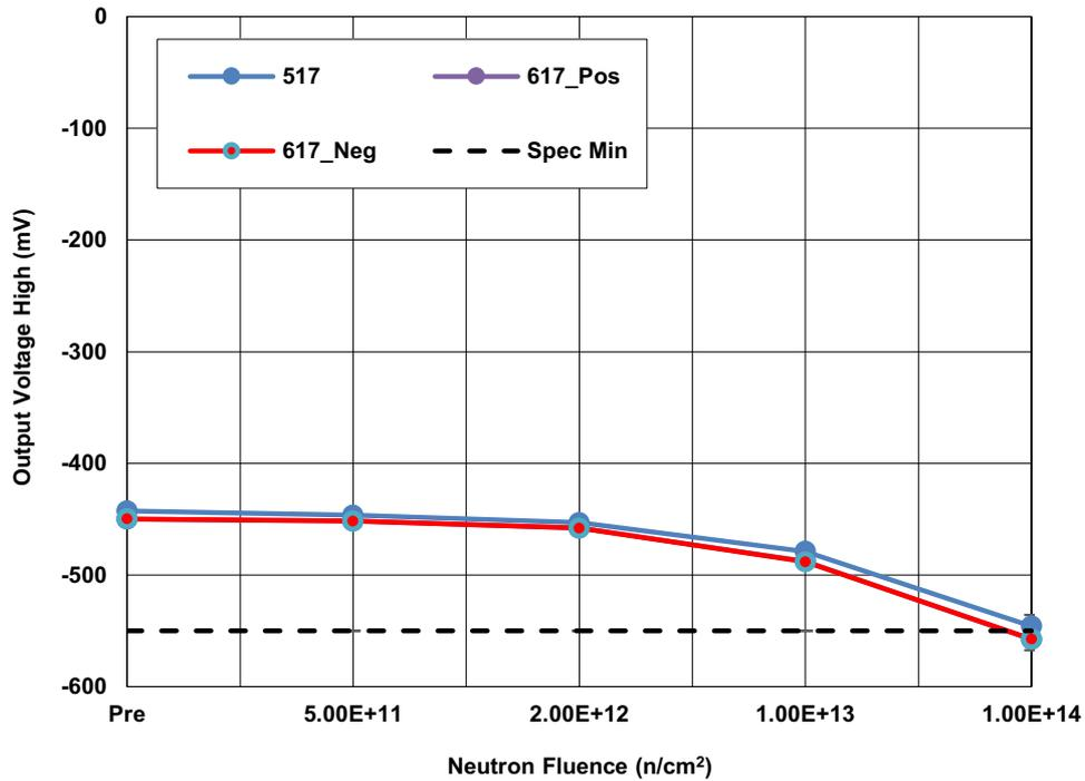
Figure 13. ISL70x17SEH high output voltage ( $V_{OH}$ ) at  $\pm 18V$  with  $I_{OUT} = -7.5mA$  following irradiation to each level. The error bars represent the minimum and maximum measured values. The SMD limit is -550mV maximum.
