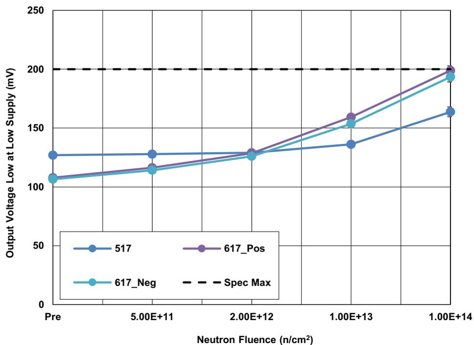
Figure 14. ISL70x17SEH low output voltage ( $V_{OLLV}$ ) with  $V_{CC} = 4V$ ,  $V_{EE} = -4V$ ,  $V_{CO} = 1.5V$ ,  $V_{EO} = -1.5V$ ,  $I_{OUT} = 1.5mA$  following irradiation to each level. The error bars represent the minimum and maximum measured values. The SMD limit is 200mV maximum.
