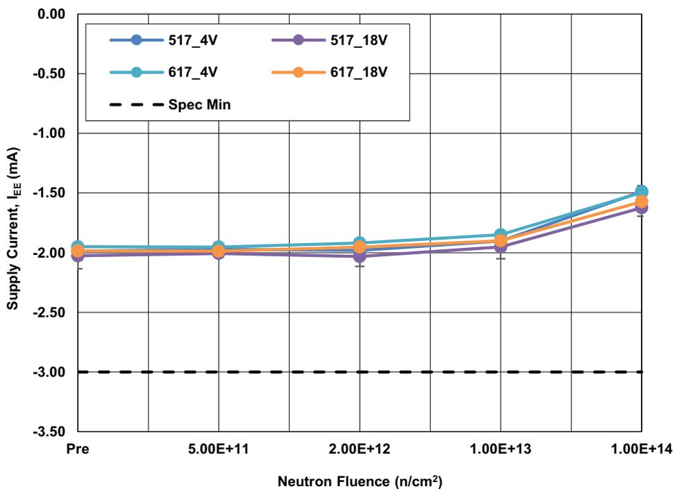
Figure 26. ISL70x17SEH supply current ( $I_{EE}$ ) at  $\pm 4V$  and  $\pm 18V$  following irradiation to each level. The error bars represent the minimum and maximum measured values. The SMD limit is -3mA minimum.
