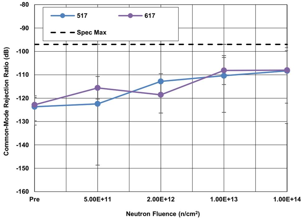
Figure 5. ISL70x17SEH common mode rejection ratio (CMRR) with Gain = 1, following irradiation to each level. The error bars represent the minimum and maximum measured values. The SMD limit is -97dB maximum.
