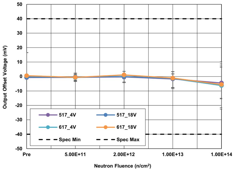
Figure 24. ISL70x17SEH output offset voltage ( $V_{OSOUT}$ ), at  $\pm 5V$  and  $\pm 18V$ , with  $R_{FB} = 120k$  following irradiation to each level. The error bars represent the minimum and maximum measured values. The SMD limits are  $-40mV$  minimum and  $40mV$  maximum.
