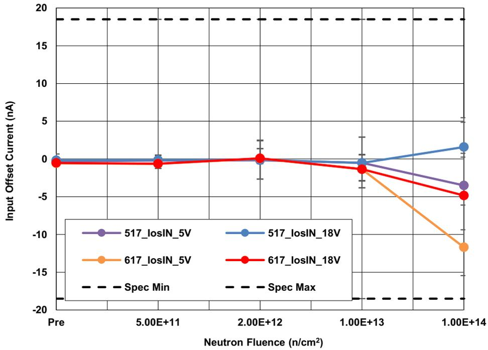
Figure 3. ISL70x17SEH input offset current ( $I_{OS}$ ) at  $\pm 5V$  and  $\pm 18V$  following irradiation to each level. The error bars represent the minimum and maximum measured values. The SMD limits are  $-18.5nA$  minimum and  $18.5nA$  maximum.
