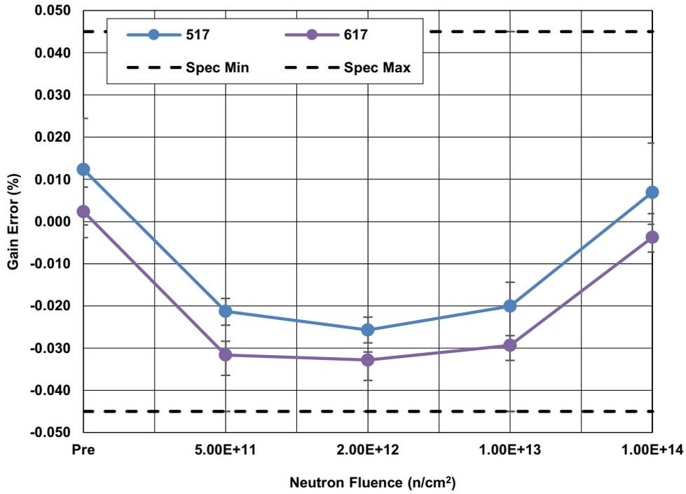
Figure 19. ISL70x17SEH gain error ( $E_G$ ) with  $V_{OUT} = \pm 10V$ ,  $RFB = 120k$ ,  $Gain = 100$  following irradiation to each level. The error bars represent the minimum and maximum measured values. The SMD limits are -0.045% minimum and 0.045% maximum.
