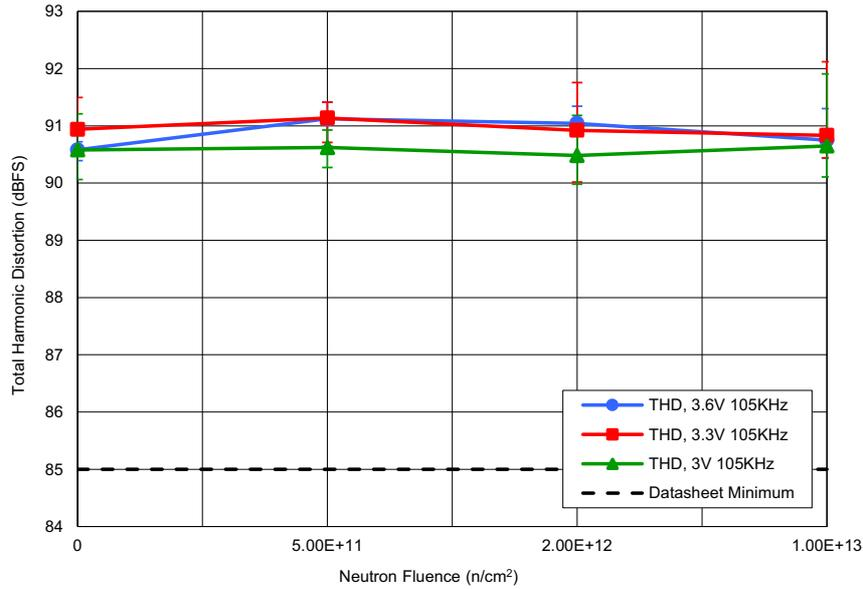
Figure 9. ISL73141SEH average total harmonic distortion (THD) with  $AV_{CC} = 3.6V, 3.3V$  and  $3.0V, DV_{CC} = 2.5V, REF = 3.0V, F_{IN} = 105kHz$  (first five harmonics), and  $A_{IN} = -1dBFS$  following irradiation to each level. The error bars (if visible) represent the minimum and maximum measured values. The post – TID irradiation datasheet limit is a minimum of 85dB.
