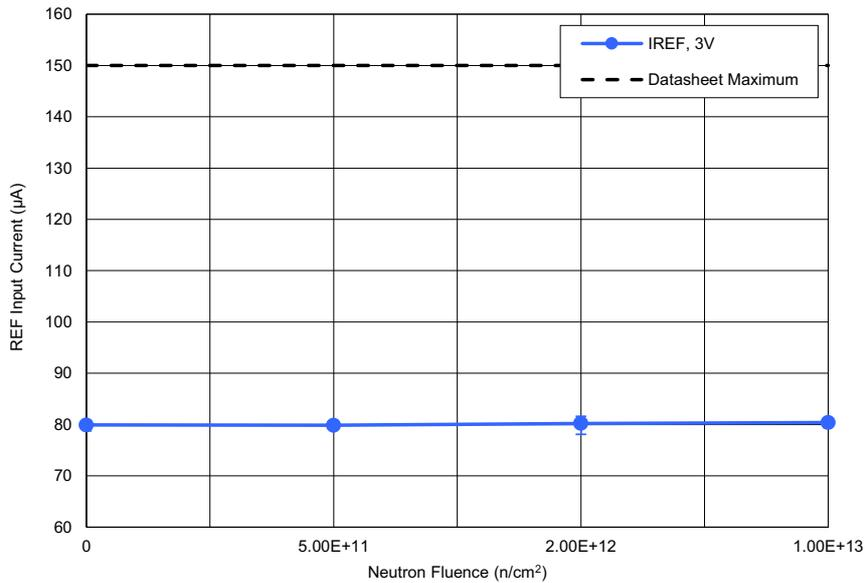
Figure 12. ISL73141SEH average REF input current ( $I_{REF}$ ) with  $AV_{CC} = 3.3V$ ,  $DV_{CC} = 2.5V$ ,  $REF = 3.0V$ ,  $f_{SAMP} = 750kps$ , and  $A_{IN} = -1dBFS$  following irradiation to each level. The error bars (if visible) represent the minimum and maximum measured values. The post – TID irradiation datashheet limit is a maximum of  $150\mu A$ .
