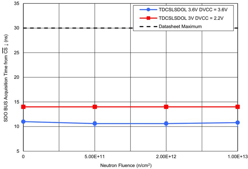
Figure 29. ISL73141SEH average SDO bus acquisition time from  $\overline{CS}$  falling edge ( $t_{DCSLSDOL}$ ) with  $AV_{CC} = 3.6V$ ,  $DV_{CC} = 3.6V$  and  $AV_{CC} = 3.0V$ ,  $DV_{CC} = 2.2V$ ,  $REF = 3.0V$ ,  $f_{SAMP} = 750ksps$ ,  $A_{IN} = -1dBFS$ , and  $C_L = 10pF$  following irradiation to each level. The error bars (if visible) represent the minimum and maximum measured values. The post – TID irradiation datasheet limit is a maximum of 30ns.
