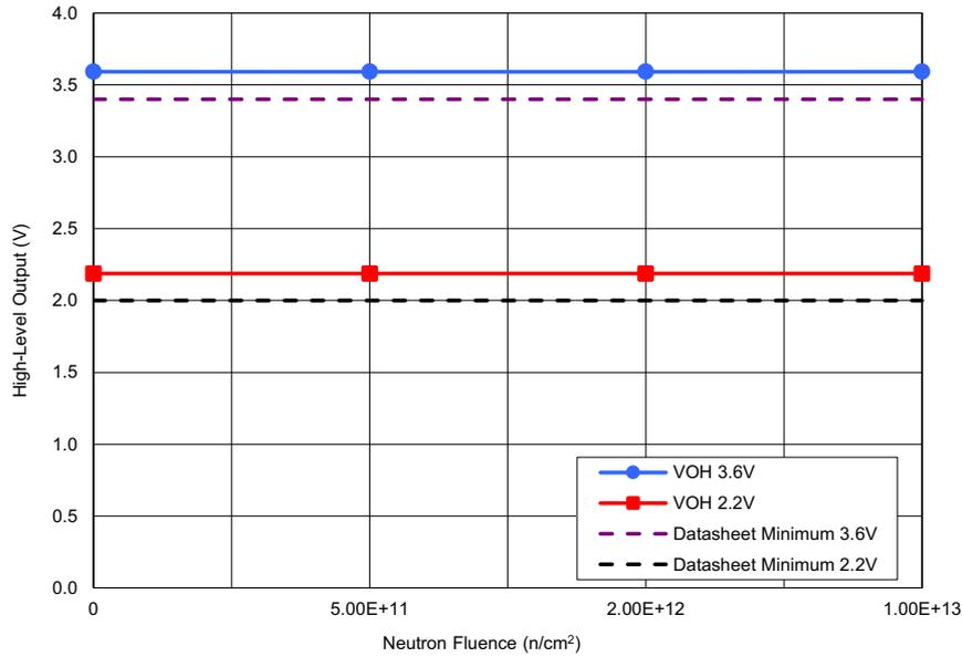
Figure 21. ISL73141SEH average high-level output (V<sub>OH</sub>) with AV<sub>CC</sub> = 3.3V, DV<sub>CC</sub> = 3.6V and 2.2V, REF = 3.0V, and I<sub>O</sub> = -500μA following irradiation to each level. The error bars (if visible) represent the minimum and maximum measured values. The post – TID irradiation datasheet limits are minimums of 3.4V for DV<sub>CC</sub> = 3.6V and 2.0V for DV<sub>CC</sub> = 2.2V.
