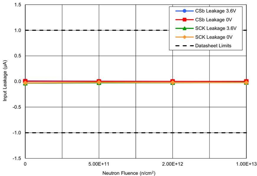
Figure 20. ISL73141SEH average input leakage current ( $I_{IN}$ ) on SCK and  $\overline{CS}$  with  $AV_{CC} = 3.3V$ ,  $DV_{CC} = 2.5V$ ,  $REF = 3.0V$ , and  $V_{IN} = 3.6V$  and  $0V$  following irradiation to each level. The error bars (if visible) represent the minimum and maximum measured values. The post – TID irradiation datasheet limits are a minimum of  $-1\mu A$  with a maximum of  $1\mu A$ .
