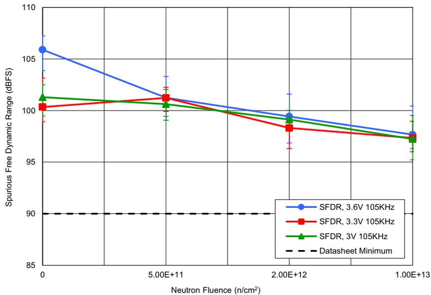
Figure 10. ISL73141SEH average spurious free dynamic range (SFDR) with  $AV_{CC} = 3.6V, 3.3V$  and  $3.0V, DV_{CC} = 2.5V, REF = 3.0V, F_{IN} = 105kHz$  (first five harmonics excluded), and  $A_{IN} = -1dBFS$  following irradiation to each level. The error bars (if visible) represent the minimum and maximum measured values. The post – TID irradiation datasheet limit is a minimum of 90dB.
