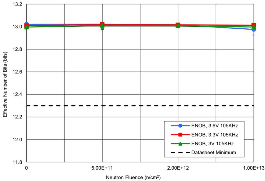
Figure 8. ISL73141SEH average effective number of bits (ENOB) with  $AV_{CC} = 3.6V, 3.3V$  and  $3.0V$ ,  $DV_{CC} = 2.5V$ ,  $REF = 3.0V$ ,  $F_{IN} = 105kHz$ , and  $A_{IN} = -1dBFS$  following irradiation to each level. The error bars (if visible) represent the minimum and maximum measured values. The post – TID irradiation datasheet limit is a minimum of 12.3bits.
