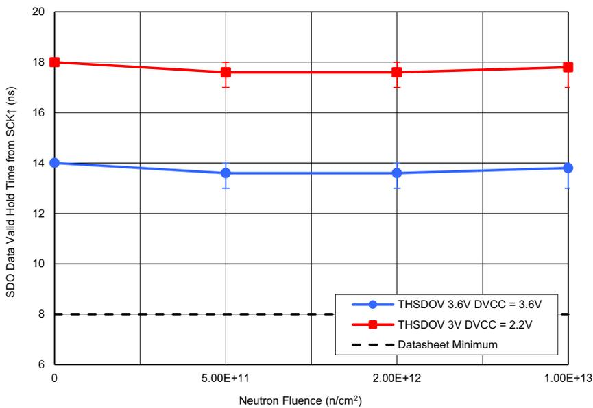
Figure 28. ISL73141SEH average SDO data valid hold time from SCK rising edge ( $t_{HSDOV}$ ) with  $AV_{CC} = 3.6V$ ,  $DV_{CC} = 3.6V$  and  $AV_{CC} = 3.0V$ ,  $DV_{CC} = 2.2V$ ,  $REF = 3.0V$ ,  $f_{SAMP} = 750ksps$ ,  $A_{IN} = -1dBFS$ , and  $C_L = 10pF$  following irradiation to each level. The error bars (if visible) represent the minimum and maximum measured values. The post – TID irradiation datasheet limit is a minimum of 8ns.
