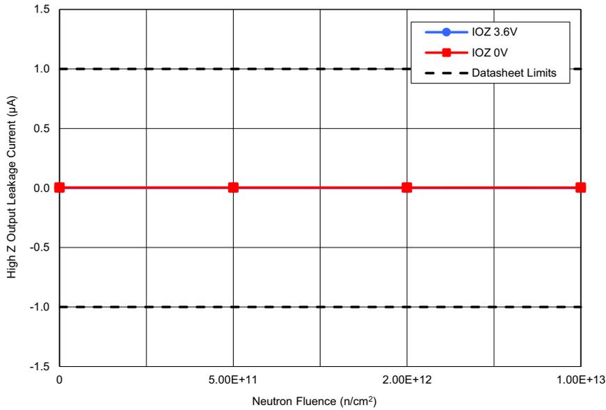
Figure 23. ISL73141SEH average Hi-Z output leakage current ( $I_{OZ}$ ) with  $AV_{CC} = 3.3V$ ,  $DV_{CC} = 3.6V$ ,  $V_{OUT} = 3.6V$  and  $0V$ , and  $REF = 3.0V$  following irradiation to each level. The error bars (if visible) represent the minimum and maximum measured values. The post – TID irradiation datasheet limits are a minimum of  $-1\mu A$  with a maximum of  $1\mu A$ .
