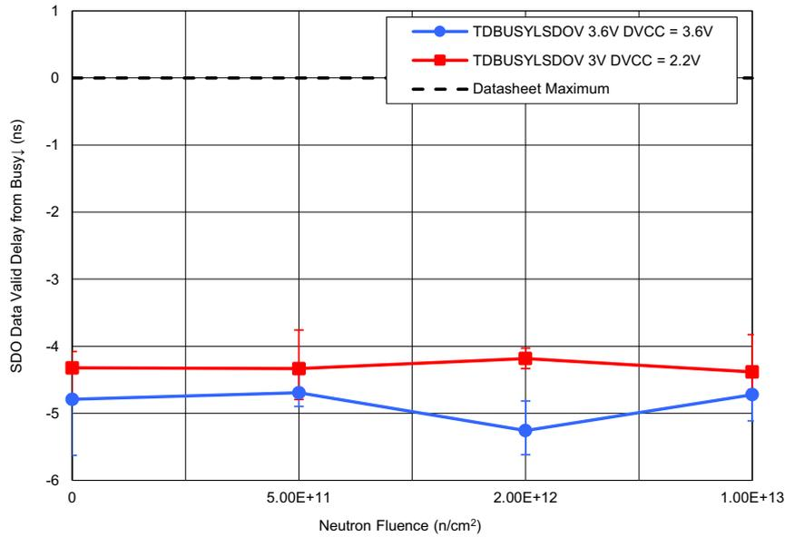
Figure 27. ISL73141SEH average SDO data valid delay from BUSY falling edge ( $t_{DBUSYLSDOV}$ ) with  $AV_{CC} = 3.6V$ ,  $DV_{CC} = 3.6V$  and  $AV_{CC} = 3.0V$ ,  $DV_{CC} = 2.2V$ ,  $REF = 3.0V$ ,  $f_{SAMP} = 750ksps$ ,  $A_{IN} = -1dBFS$ , and  $C_L = 10pF$  following irradiation to each level. The error bars (if visible) represent the minimum and maximum measured values. The post – TID irradiation datasheet limit is a maximum of 0ns.
