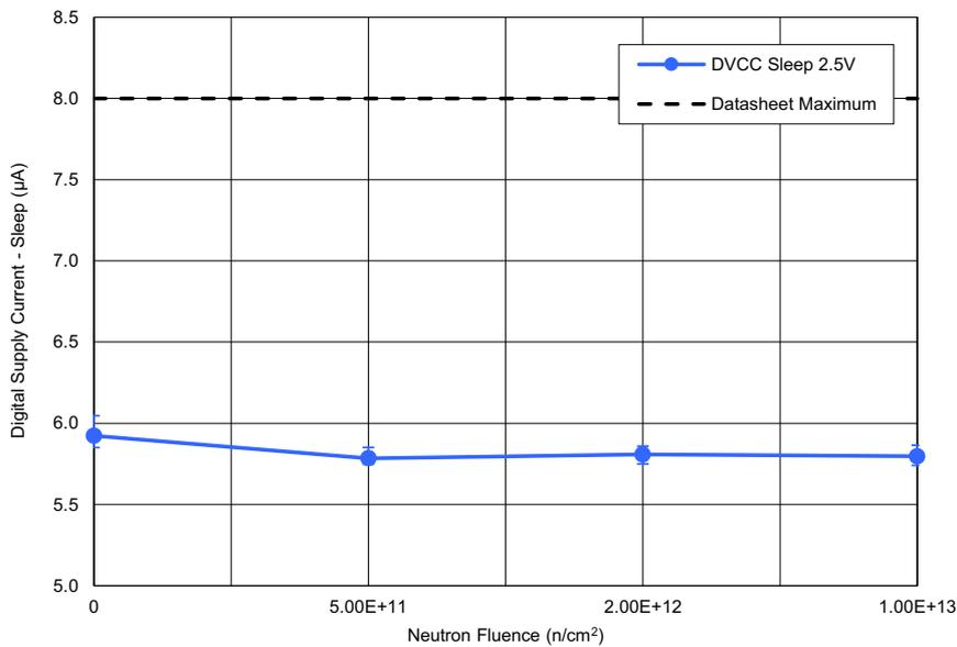
Figure 18. ISL73141SEH average digital supply current – sleep ( $I_{SLDVCC}$ ) with  $AV_{CC} = 3.3V$ ,  $DV_{CC} = 2.5V$ ,  $REF = 3.0V$ , and  $PD = GND$  following irradiation to each level. The error bars (if visible) represent the minimum and maximum measured values. The post – TID irradiation datasheet limit is a maximum of  $8\mu A$ .
