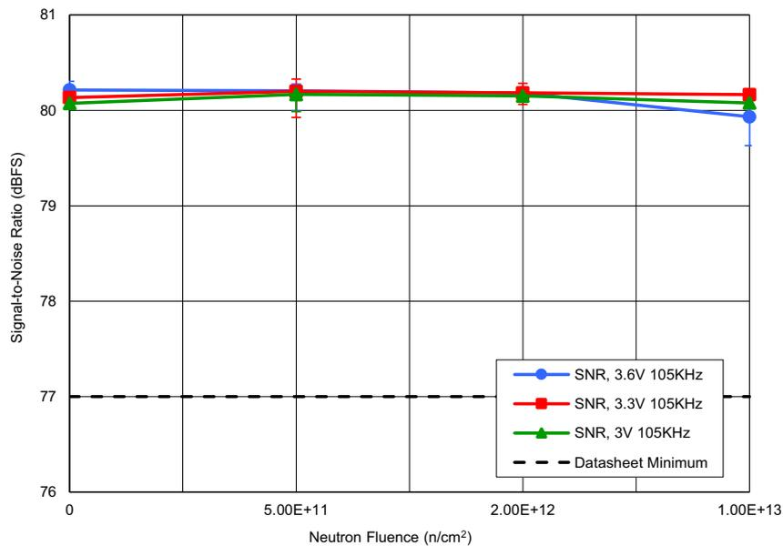
Figure 6. ISL73141SEH average signal-to-noise ratio (SNR) with  $AV_{CC} = 3.6V$ ,  $3.3V$  and  $3.0V$ ,  $DV_{CC} = 2.5V$ ,  $REF = 3.0V$ ,  $F_{IN} = 105kHz$ , and  $A_{IN} = -1dBFS$  following irradiation to each level. The error bars (if visible) represent the minimum and maximum measured values. The post – TID irradiation datasheet limit is a minimum of 77dB.
