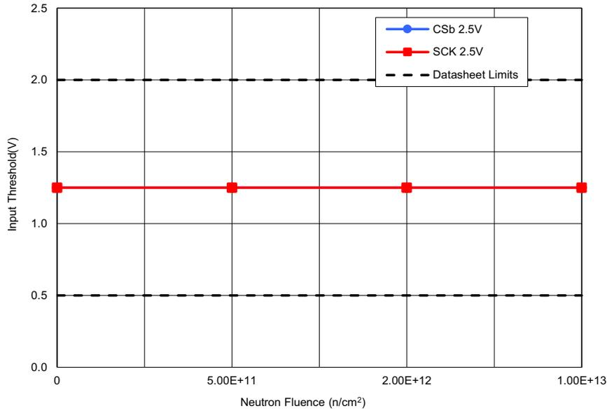
Figure 19. ISL73141SEH average high-level input ( $V_{IH}$ ) and low-level input ( $V_{IL}$ ) with  $AV_{CC} = 3.3V$ ,  $DV_{CC} = 2.5V$ , and  $REF = 3.0V$  following irradiation to each level. The error bars (if visible) represent the minimum and maximum measured values. The post – TID irradiation datasheet limits are a 2.0V minimum for  $V_{IH}$  and a 0.5V maximum for  $V_{IL}$ .
