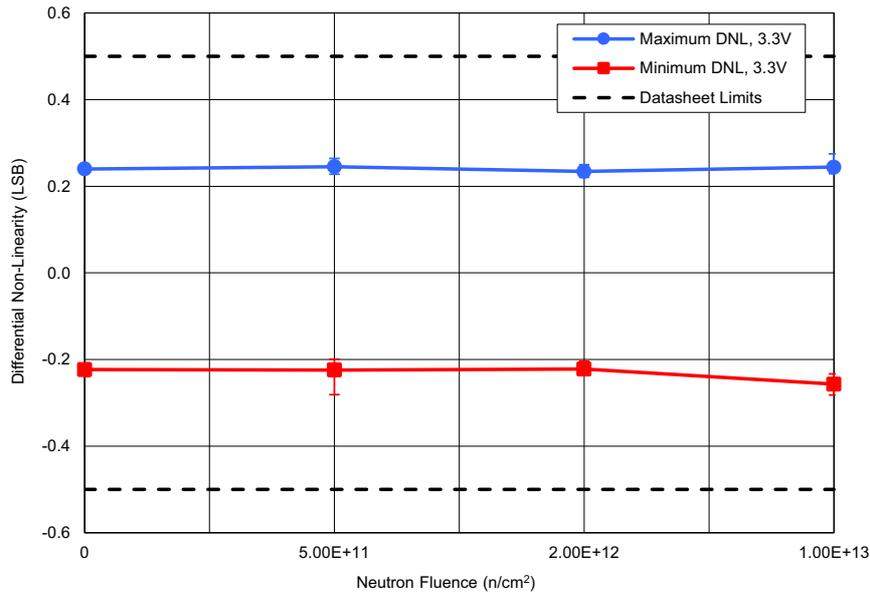
Figure 3. ISL73141SEH average minimum and maximum differential non-linearity (DNL) with  $AV_{CC} = 3.3V$ ,  $DV_{CC} = 2.5V$ ,  $REF = 3.0V$ ,  $f_{SAMP} = 750ksps$ , and  $A_{IN} =$  full-scale sine wave following irradiation to each level. The error bars (if visible) represent the minimum and maximum measured values. The post – TID irradiation datasheet limits are a minimum of -0.5LSB with a maximum of 0.5LSB.
