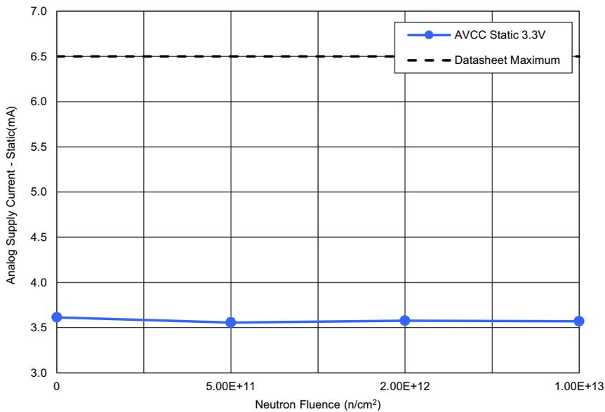
Figure 14. ISL73141SEH average analog supply current – static ( $I_{STATIC}$ ) with  $AV_{CC} = 3.3V$ ,  $DV_{CC} = 2.5V$ ,  $REF = 3.0V$ , and  $CS = DV_{CC}$  following irradiation to each level. The error bars (if visible) represent the minimum and maximum measured values. The post – TID irradiation datasheet limit is a maximum of 6.5mA.
