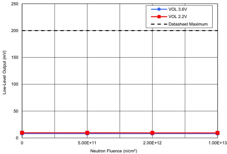
Figure 22. ISL73141SEH average low-level output (V<sub>OL</sub>) with AV<sub>CC</sub> = 3.3V, DV<sub>CC</sub> = 3.6V and 2.2V, REF = 3.0V, and I<sub>O</sub> = 500μA following irradiation to each level. The error bars (if visible) represent the minimum and maximum measured values. The post – TID irradiation datasheet limit is a maximum of 200mV.
