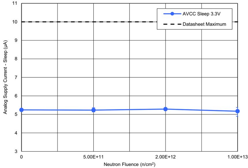
Figure 15. ISL73141SEH average analog supply current – sleep ( $I_{SLAVCC}$ ) with  $AV_{CC} = 3.3V$ ,  $DV_{CC} = 2.5V$ ,  $REF = 3.0V$ , and  $PD = GND$  following irradiation to each level. The error bars (if visible) represent the minimum and maximum measured values. The post – TID irradiation datasheet limit is a maximum of  $10\mu A$ .
