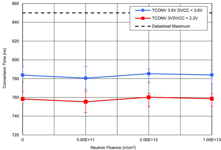
Figure 25. ISL73141SEH average conversion time ( $t_{CONV}$ ) with  $AV_{CC} = 3.6V$ ,  $DV_{CC} = 3.6V$  and  $AV_{CC} = 3.0V$ ,  $DV_{CC} = 2.2V$ ,  $REF = 3.0V$ ,  $f_{SAMP} = 750ksps$ , and  $A_{IN} = -1dBFS$  following irradiation to each level. The error bars (if visible) represent the minimum and maximum measured values. The post – TID irradiation datasheet limit is a maximum of 850ns.
