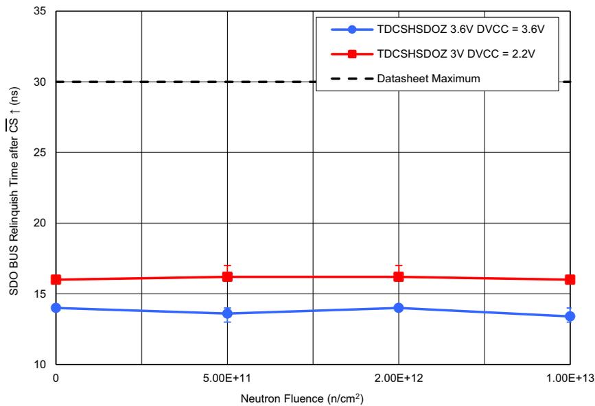
Figure 30. ISL73141SEH average SDO bus relinquish time after  $\overline{CS}$  raising edge ( $t_{DCSHSDOZ}$ ) with  $AV_{CC} = 3.6V$ ,  $DV_{CC} = 3.6V$  and  $AV_{CC} = 3.0V$ ,  $DV_{CC} = 2.2V$ ,  $REF = 3.0V$ ,  $f_{SAMP} = 750ksps$ ,  $A_{IN} = -1dBFS$ , and  $C_L = 10pF$  following irradiation to each level. The error bars (if visible) represent the minimum and maximum measured values. The post – TID irradiation datasheet limit is a maximum of 30ns.
