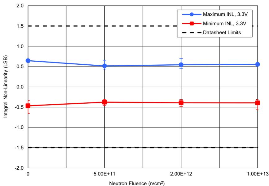
Figure 2. ISL73141SEH average minimum and maximum integral non-linearity (INL) with AV<sub>CC</sub> = 3.3V, DV = 2.5V, REF = 3.0V, f<sub>SAMP</sub> = 750ksps, and A<sub>IN</sub> = full-scale sine wave following irradiation to each level. The error bars (if visible) represent the minimum and maximum measured values. The post – TID irradiation datasheet limits are a minimum of -1.5LSB with a maximum of 1.5LSB.
