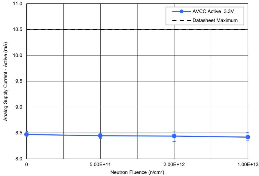
Figure 13. ISL73141SEH average analog supply current – active ( $I_{AVCC}$ ) with  $AV_{CC} = 3.3V$ ,  $DV_{CC} = 2.5V$ ,  $REF = 3.0V$ ,  $f_{SAMP} = 750ksps$ , and  $A_{IN} = -1dBFS$  following irradiation to each level. The error bars (if visible) represent the minimum and maximum measured values. The post – TID irradiation datasheet limit is a maximum of 10.5mA.
