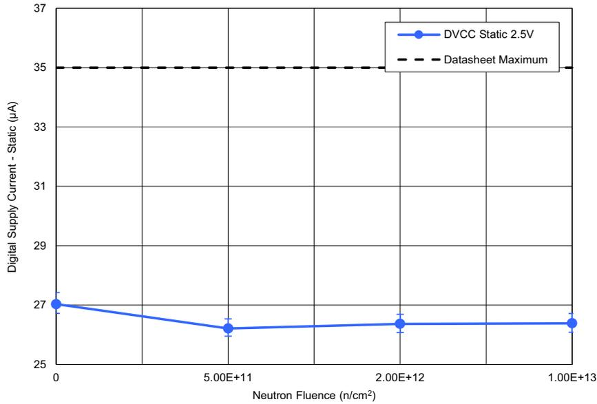
Figure 17. ISL73141SEH average digital supply current – static ( $I_{STDVCC}$ ) with  $AV_{CC} = 3.3V$ ,  $DV_{CC} = 2.5V$ ,  $REF = 3.0V$ , and  $CS = DV_{CC}$  following irradiation to each level. The error bars (if visible) represent the minimum and maximum measured values. The post – TID irradiation datasheet limit is a maximum of  $35\mu A$ .
