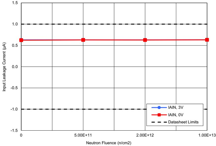
Figure 11. ISL73141SEH average input leakage current ( $I_{AIN}$ ) with  $AV_{CC} = 3.3V$ ,  $DV_{CC} = 2.5V$ ,  $REF = 3.0V$ ,  $f_{SAMP} = 750kps$ , and  $A_{IN} = 3.0V$  and  $0V$  following irradiation to each level. The error bars (if visible) represent the minimum and maximum measured values. The post – TID irradiation datashheet limits are a minimum of  $-1\mu A$  with a maximum of  $1\mu A$ .
