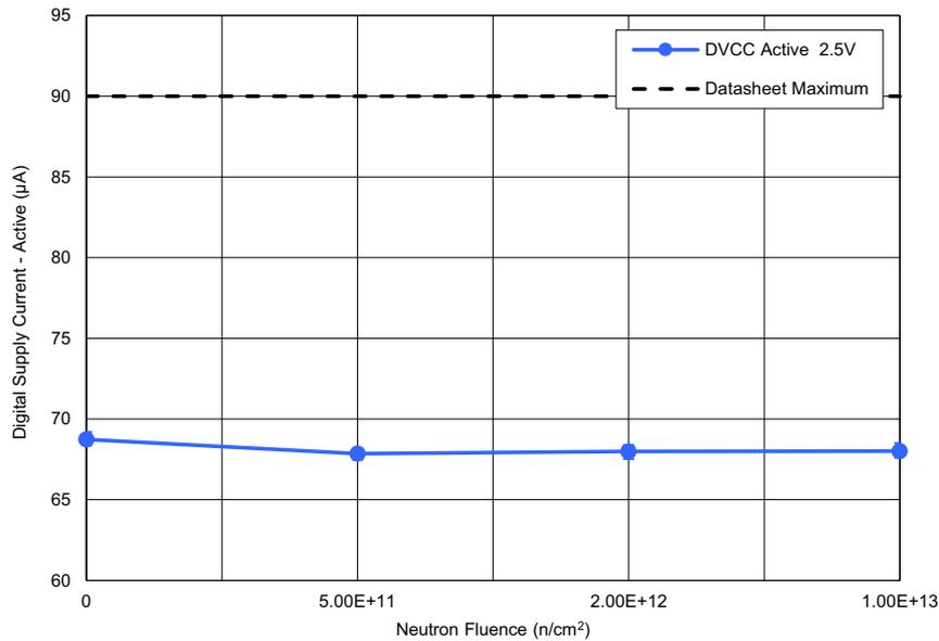
Figure 16. ISL73141SEH average digital supply current – active ( $I_{DVCC}$ ) with  $AV_{CC} = 3.3V$ ,  $DV_{CC} = 2.5V$ ,  $REF = 3.0V$ ,  $f_{SCK} = 33MHz$ , and  $C_L = 10pF$  following irradiation to each level. The error bars (if visible) represent the minimum and maximum measured values. The post – TID irradiation datasheet limit is a maximum of  $90\mu A$ .
