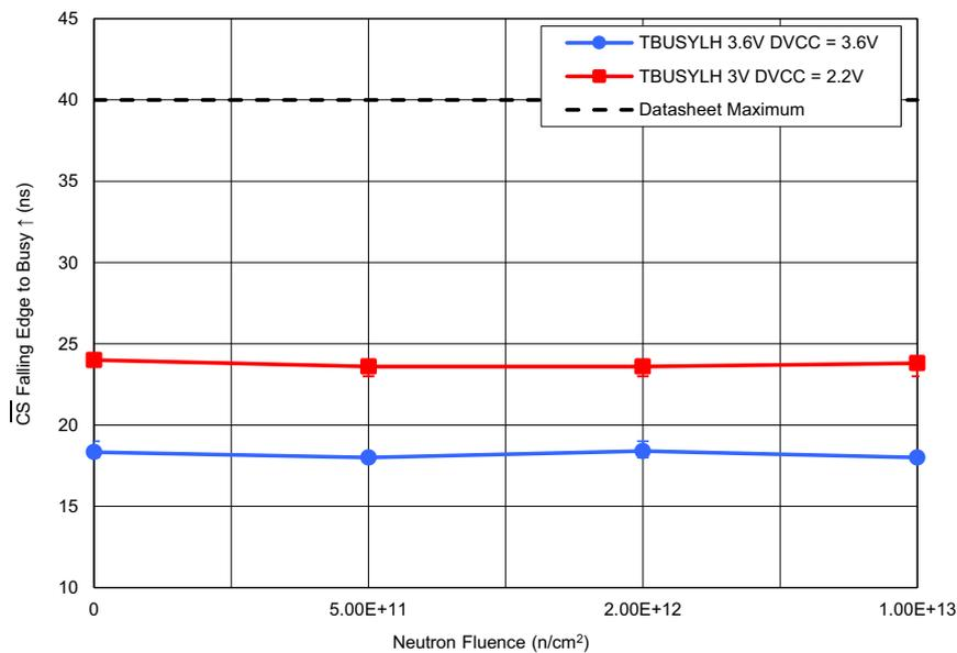
Figure 26. ISL73141SEH average  $\overline{CS}$  falling edge to BUSY rising edge ( $t_{BUSYLH}$ ) with  $AV_{CC} = 3.6V$ ,  $DV_{CC} = 3.6V$  and  $AV_{CC} = 3.0V$ ,  $DV_{CC} = 2.2V$ ,  $REF = 3.0V$ ,  $f_{SAMP} = 750ksps$ ,  $A_{IN} = -1dBFS$ , and  $C_L = 10pF$  following irradiation to each level. The error bars (if visible) represent the minimum and maximum measured values. The post – TID irradiation datasheet limit is a maximum of 40ns.
