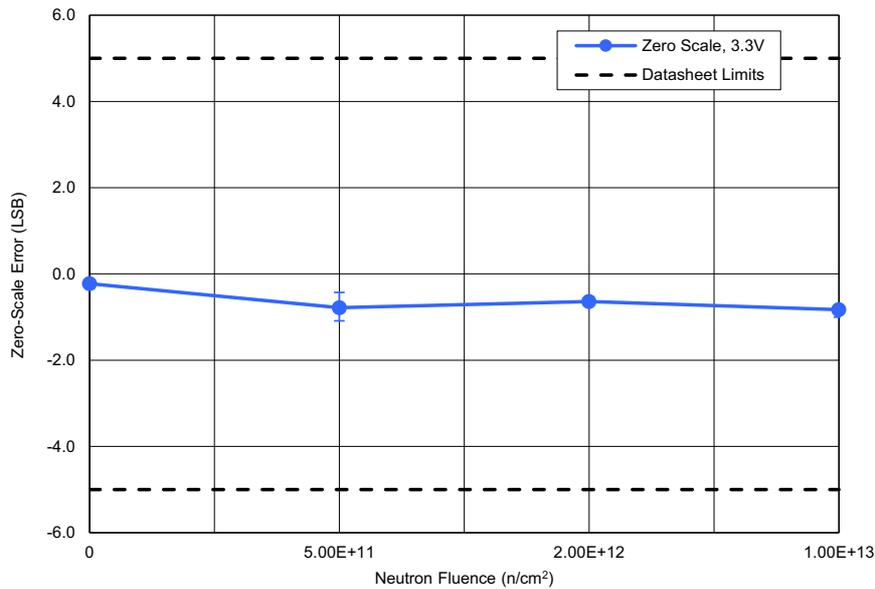
Figure 4. ISL73141SEH average zero scale error (VOFF) with  $AV_{CC} = 3.3V$ ,  $DV_{CC} = 2.5V$ ,  $REF = 3.0V$ ,  $f_{SAMP} = 750ksps$ , and  $A_{IN} = GND$  following irradiation to each level. The error bars (if visible) represent the minimum and maximum measured values. The post – TID irradiation datasheet limits are a minimum of -5LSB with a maximum of 5LSB.
