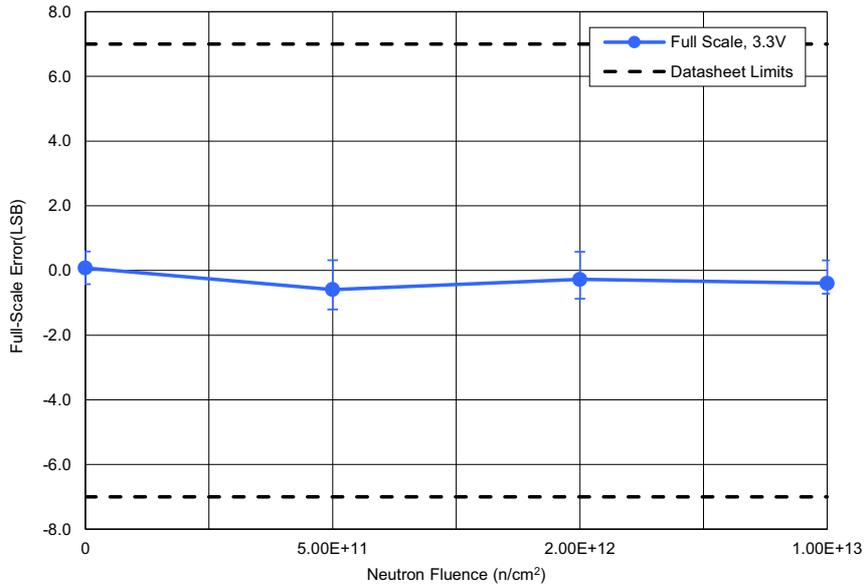
Figure 5. ISL73141SEH average full-scale error (FSE) with  $AV_{CC} = 3.3V$ ,  $DV_{CC} = 2.5V$ ,  $REF = 3.0V$ ,  $f_{SAMP} = 750ksps$ , and  $A_{IN} = VREF$  following irradiation to each level. The error bars (if visible) represent the minimum and maximum measured values. The post – TID irradiation datasheet limits are a minimum of -7LSB with a maximum of 7LSB.
