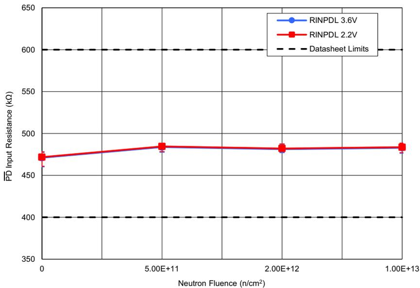
Figure 24. ISL73141SEH average  $\overline{PD}$  input resistance ( $R_{INPDL}$ ) with  $AV_{CC} = 3.3V$ ,  $DV_{CC} = 3.6V$  and  $2.2V$ , and  $REF = 3.0V$  following irradiation to each level. The error bars (if visible) represent the minimum and maximum measured values. The post – TID irradiation datasheet limits are a minimum of  $400k\Omega$  with a maximum of  $600k\Omega$ .
