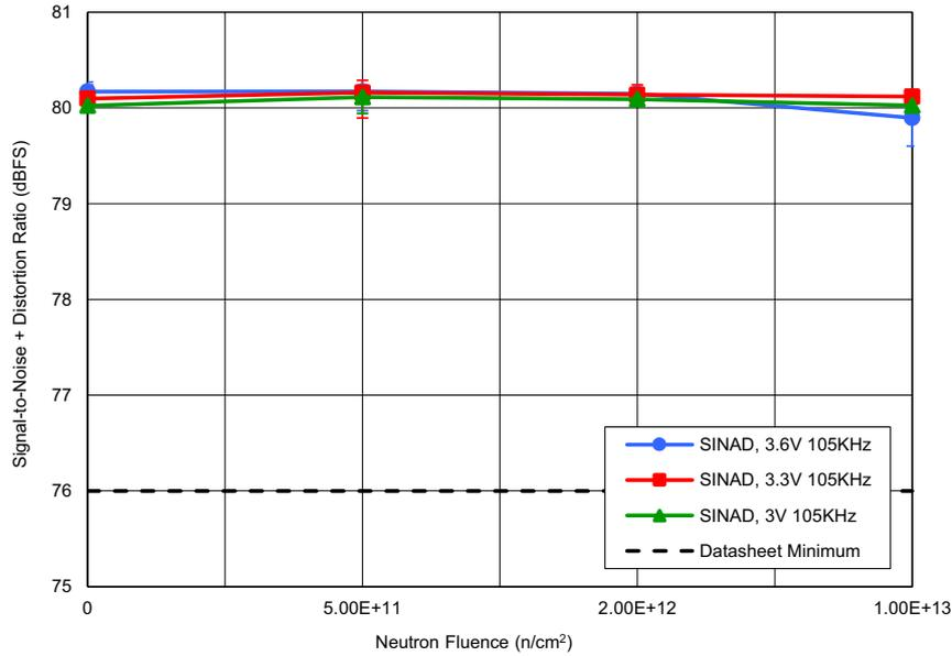
Figure 7. ISL73141SEH average signal-to-noise + distortion ratio (SINAD) with  $AV_{CC} = 3.6V, 3.3V$  and  $3.0V$ ,  $DV_{CC} = 2.5V$ ,  $REF = 3.0V$ ,  $F_{IN} = 105kHz$ , and  $A_{IN} = -1dBFS$  following irradiation to each level. The error bars (if visible) represent the minimum and maximum measured values. The post – TID irradiation datasheet limit is a minimum of 76dB.
