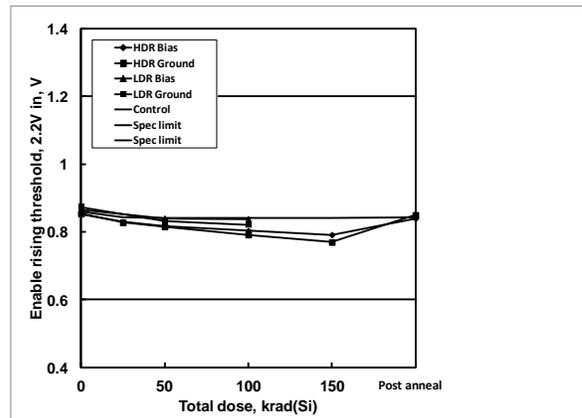
**Figure 5:** ISL75051SEH enable rising threshold, 2.2V input, as a function of biased and grounded high and low dose rate irradiation and subsequent high temperature accelerated post-high dose rate aging at 100°C. The dose rate was 80 rad(Si)/s. Sample size was 6 for the high dose rate cells and 4 for the low dose rate cells, and three control units were used for the high dose rate test. The specification limits are 0.600V – 1.200V.
