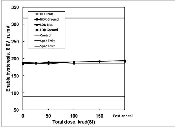
**Figure 10:** ISL75051SEH enable hysteresis, 6.0V input, as a function of biased and grounded high and low dose rate irradiation and subsequent high temperature accelerated post-high dose rate aging at 100°C. The dose rate was 80 rad(Si)/s. Sample size was 6 for the high dose rate cells and 4 for the low dose rate cells, and three control units were used for the high dose rate test. The specification limits are 90.0mV – 318.0mV.
