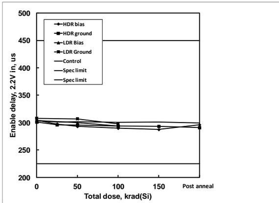
**Figure 11:** ISL75051SEH enable propagation delay, 2.2V input, as a function of biased and grounded high and low dose rate irradiation and subsequent high temperature accelerated post-high dose rate aging at 100°C. The dose rate was 80 rad(Si)/s. Sample size was 6 for the high dose rate cells and 4 for the low dose rate cells, and three control units were used for the high dose rate test. The specification limits are 225μs – 450μs.
