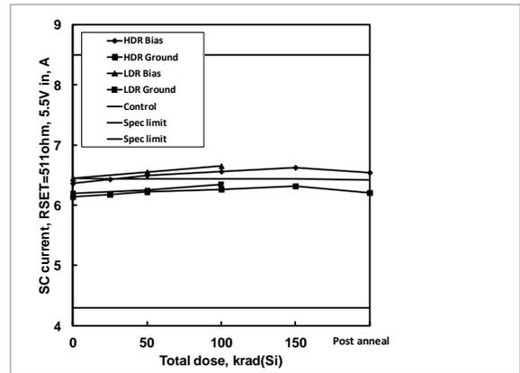
**Figure 56:** ISL75051SEH output short circuit current, RSET=511Ω, 6.0V in, as a function of biased and grounded high and low dose rate irradiation and subsequent high temperature accelerated post-high dose rate aging at 100°C. The dose rate was 80 rad(Si)/s. Sample size was 6 for the high dose rate cells and 4 for the low dose rate cells, and three control units were used for the high dose rate test. The specification limits are 4.300A to 8.500A.
