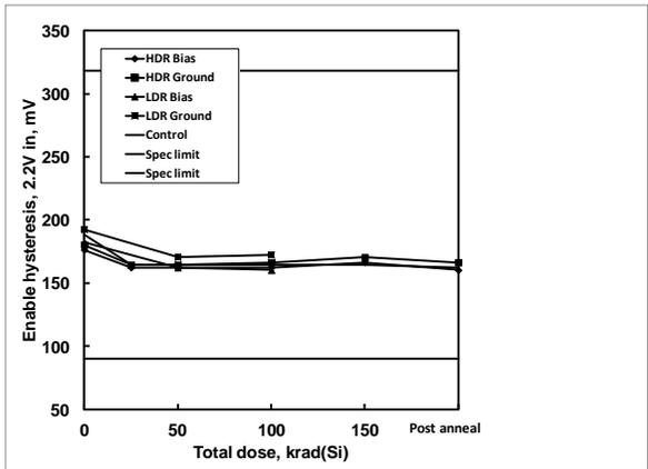
**Figure 7:** ISL75051SEH enable hysteresis, 2.2V input, as a function of biased and grounded high and low dose rate irradiation and subsequent high temperature accelerated post-high dose rate aging at 100°C. The dose rate was 80 rad(Si)/s. Sample size was 6 for the high dose rate cells and 4 for the low dose rate cells, and three control units were used for the high dose rate test. The specification limits are 90.0mV – 318.0mV.
