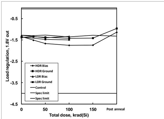
**Figure 31:** ISL75051SEH load regulation, 1.8V out, as a function of biased and grounded high and low dose rate irradiation and subsequent high temperature accelerated post-high dose rate aging at 100°C. The dose rate was 80 rad(Si)/s. Sample size was 6 for the high dose rate cells and 4 for the low dose rate cells, and three control units were used for the high dose rate test. The specification limits are -4.000mV to -0.050mV.
