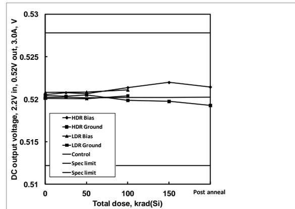
**Figure 13:** ISL75051SEH DC output voltage, 0.52V output, 2.2V input, 3A load, as a function of biased and grounded high and low dose rate irradiation and subsequent high temperature accelerated post-high dose rate aging at 100°C. The dose rate was 80 rad(Si)/s. Sample size was 6 for the high dose rate cells and 4 for the low dose rate cells, and three control units were used for the high dose rate test. The specification limits are 0.5122V – 0.5278V.
