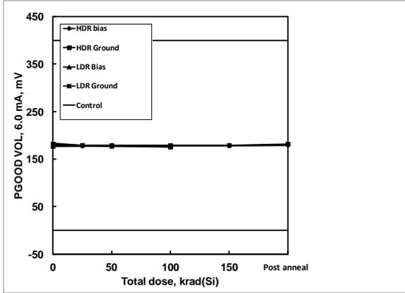
**Figure 42:** ISL75051SEH PGOOD output LOW voltage, 6mA, as a function of biased and grounded high and low dose rate irradiation and subsequent high temperature accelerated post-high dose rate aging at 100°C. The dose rate was 80 rad(Si)/s. Sample size was 6 for the high dose rate cells and 4 for the low dose rate cells, and three control units were used for the high dose rate test. The specification limits are 0mV to 400.0mV.
