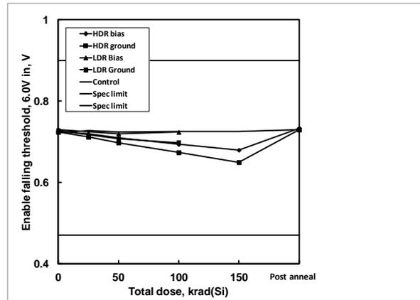
**Figure 9:** ISL75051SEH enable falling threshold, 6.0V input, as a function of biased and grounded high and low dose rate irradiation and subsequent high temperature accelerated post-high dose rate aging at 100°C. The dose rate was 80 rad(Si)/s. Sample size was 6 for the high dose rate cells and 4 for the low dose rate cells, and three control units were used for the high dose rate test. The specification limits are 0.470V – 0.900V.
