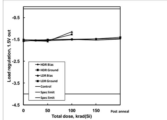
**Figure 29:** ISL75051SEH load regulation, 1.5V out, as a function of biased and grounded high and low dose rate irradiation and subsequent high temperature accelerated post-high dose rate aging at 100°C. The dose rate was 80 rad(Si)/s. Sample size was 6 for the high dose rate cells and 4 for the low dose rate cells, and three control units were used for the high dose rate test. The specification limits are -4.000mV to -0.100mV.
