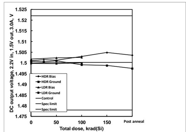
**Figure 17:** ISL75051SEH DC output voltage, 1.5V output, 2.2V input, 3A load, as a function of biased and grounded high and low dose rate irradiation and subsequent high temperature accelerated post-high dose rate aging at 100°C. The dose rate was 80 rad(Si)/s. Sample size was 6 for the high dose rate cells and 4 for the low dose rate cells, and three control units were used for the high dose rate test. The specification limits are 1.4780V – 1.5220V.
