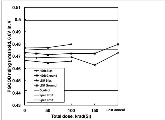
**Figure 43:** ISL75051SEH PGOOD rising threshold, 6.0V in, as a function of biased and grounded high and low dose rate irradiation and subsequent high temperature accelerated post-high dose rate aging at 100°C. The dose rate was 80 rad(Si)/s. Sample size was 6 for the high dose rate cells and 4 for the low dose rate cells, and three control units were used for the high dose rate test. The specification limits are 0.4264V to 0.4836V.
