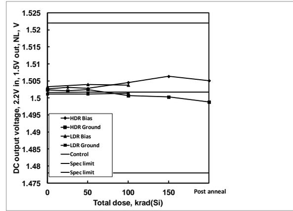
**Figure 16:** ISL75051SEH DC output voltage, 1.5V output, 2.2V input, no load, as a function of biased and grounded high and low dose rate irradiation and subsequent high temperature accelerated post-high dose rate aging at 100°C. The dose rate was 80 rad(Si)/s. Sample size was 6 for the high dose rate cells and 4 for the low dose rate cells, and three control units were used for the high dose rate test. The specification limits are 1.4780V – 1.5220V.
