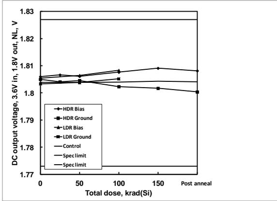
**Figure 22:** ISL75051SEH DC output voltage, 1.8V output, 3.6V input, no load, as a function of biased and grounded high and low dose rate irradiation and subsequent high temperature accelerated post-high dose rate aging at 100°C. The dose rate was 80 rad(Si)/s. Sample size was 6 for the high dose rate cells and 4 for the low dose rate cells, and three control units were used for the high dose rate test. The specification limits are 1.7730V – 1.8270V.
