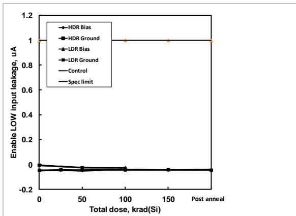
**Figure 3:** ISL75051SEH enable HIGH input current as a function of biased and grounded high and low dose rate irradiation and subsequent high temperature accelerated post-high dose rate aging at 100°C. The dose rate was 80 rad(Si)/s. Sample size was 6 for the high dose rate cells and 4 for the low dose rate cells, and three control units were used for the high dose rate test. The specification limits are -0.100µA – +1.000µA.
