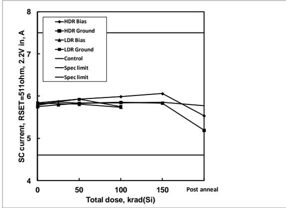
**Figure 54:** ISL75051SEH output short circuit current, RSET=511Ω, 2.2V in, as a function of biased and grounded high and low dose rate irradiation and subsequent high temperature accelerated post-high dose rate aging at 100°C. The dose rate was 80 rad(Si)/s. Sample size was 6 for the high dose rate cells and 4 for the low dose rate cells, and three control units were used for the high dose rate test. The specification limits are 4.600A to 7.500A.
