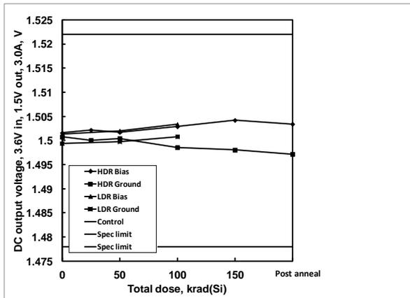
**Figure 19:** ISL75051SEH DC output voltage, 1.5V output, 3.6V input, 3A load, as a function of biased and grounded high and low dose rate irradiation and subsequent high temperature accelerated post-high dose rate aging at 100°C. The dose rate was 80 rad(Si)/s. Sample size was 6 for the high dose rate cells and 4 for the low dose rate cells, and three control units were used for the high dose rate test. The specification limits are 1.4780V – 1.5220V.
