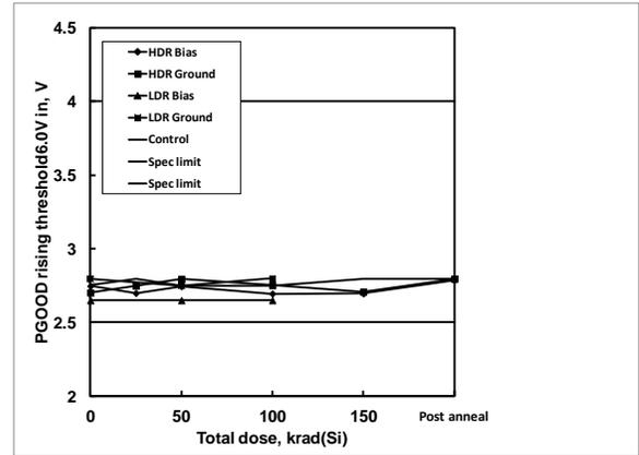
**Figure 48:** ISL75051SEH PGOOD hysteresis, 2.2V in, as a function of biased and grounded high and low dose rate irradiation and subsequent high temperature accelerated post-high dose rate aging at 100°C. The dose rate was 80 rad(Si)/s. Sample size was 6 for the high dose rate cells and 4 for the low dose rate cells, and three control units were used for the high dose rate test. The specification limits are 2.500% to 4.000%.
