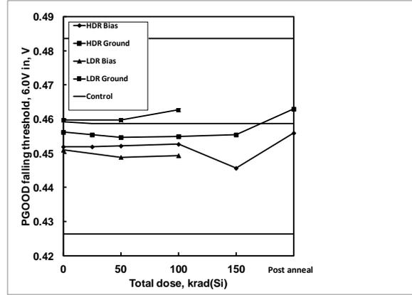
**Figure 44:** ISL75051SEH PGOOD falling threshold, 6.0V in, as a function of biased and grounded high and low dose rate irradiation and subsequent high temperature accelerated post-high dose rate aging at 100°C. The dose rate was 80 rad(Si)/s. Sample size was 6 for the high dose rate cells and 4 for the low dose rate cells, and three control units were used for the high dose rate test. The specification limits are 0.4420V to 0.492V.
