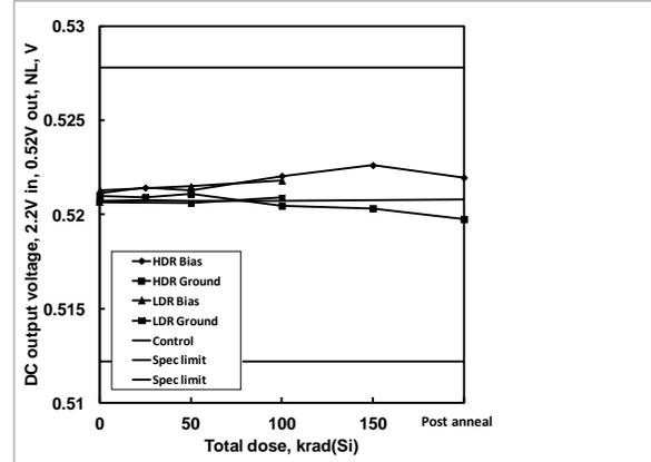
**Figure 12:** ISL75051SEH DC output voltage, 0.52V output, 2.2V input, no load, as a function of biased and grounded high and low dose rate irradiation and subsequent high temperature accelerated post-high dose rate aging at 100°C. The dose rate was 80 rad(Si)/s. Sample size was 6 for the high dose rate cells and 4 for the low dose rate cells, and three control units were used for the high dose rate test. The specification limits are 0.5122V – 0.5278V.
