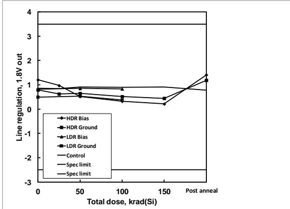
**Figure 30:** ISL75051SEH line regulation, 1.8V out, as a function of biased and grounded high and low dose rate irradiation and subsequent high temperature accelerated post-high dose rate aging at 100°C. The dose rate was 80 rad(Si)/s. Sample size was 6 for the high dose rate cells and 4 for the low dose rate cells, and three control units were used for the high dose rate test. The specification limits are -2.500mV to +3.500mV.
