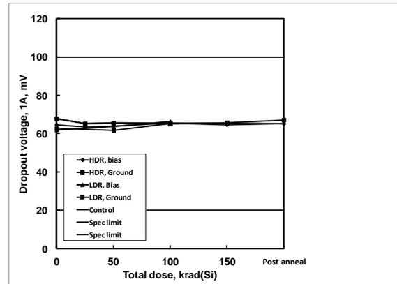
**Figure 49:** ISL75051SEH dropout voltage, 2.5V out, 1A load current, as a function of biased and grounded high and low dose rate irradiation and subsequent high temperature accelerated post-high dose rate aging at 100°C. The dose rate was 80 rad(Si)/s. Sample size was 6 for the high dose rate cells and 4 for the low dose rate cells, and three control units were used for the high dose rate test. The specification limits are 20.000mV to 100.000mV.
