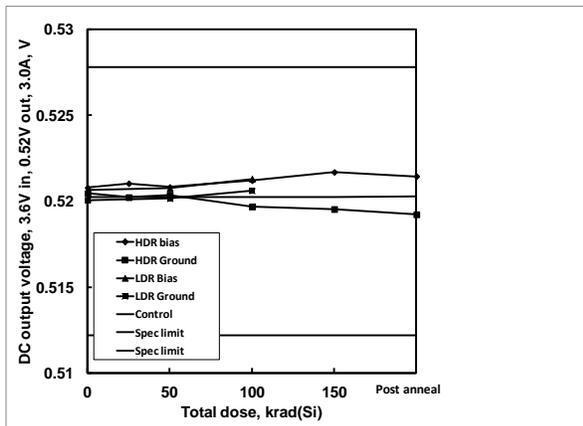
**Figure 15:** ISL75051SEH DC output voltage, 0.52V output, 3.6V input, 3A load, as a function of biased and grounded high and low dose rate irradiation and subsequent high temperature accelerated post-high dose rate aging at 100°C. The dose rate was 80 rad(Si)/s. Sample size was 6 for the high dose rate cells and 4 for the low dose rate cells, and three control units were used for the high dose rate test. The specification limits are 0.5122V – 0.5278V.
