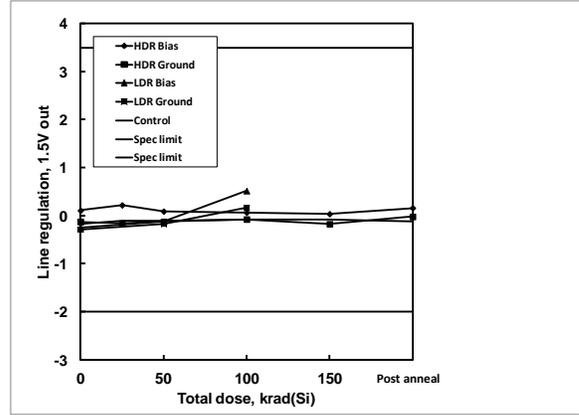
**Figure 28:** ISL75051SEH line regulation, 1.5V out, as a function of biased and grounded high and low dose rate irradiation and subsequent high temperature accelerated post-high dose rate aging at 100°C. The dose rate was 80 rad(Si)/s. Sample size was 6 for the high dose rate cells and 4 for the low dose rate cells, and three control units were used for the high dose rate test. The specification limits are -2.000mV – 3.500mV.
