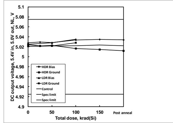
**Figure 24:** ISL75051SEH DC output voltage, 5.0V output, 5.4V input, 3A load, as a function of biased and grounded high and low dose rate irradiation and subsequent high temperature accelerated post-high dose rate aging at 100°C. The dose rate was 80 rad(Si)/s. Sample size was 6 for the high dose rate cells and 4 for the low dose rate cells, and three control units were used for the high dose rate test. The specification limits are 4.9250V – 5.0750V.
