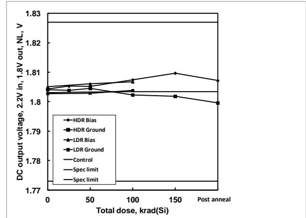
**Figure 20:** ISL75051SEH DC output voltage, 1.8V output, 2.2V input, no load, as a function of biased and grounded high and low dose rate irradiation and subsequent high temperature accelerated post-high dose rate aging at 100°C. The dose rate was 80 rad(Si)/s. Sample size was 6 for the high dose rate cells and 4 for the low dose rate cells, and three control units were used for the high dose rate test. The specification limits are 1.7730V – 1.8270V.
