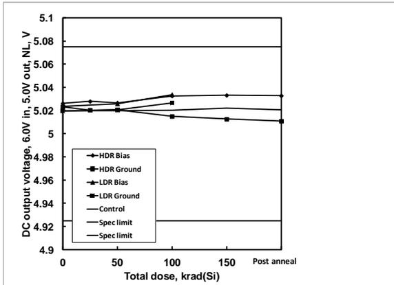
**Figure 27:** ISL75051SEH DC output voltage, 5.0V output, 6.0V input, 3A load, as a function of biased and grounded high and low dose rate irradiation and subsequent high temperature accelerated post-high dose rate aging at 100°C. The dose rate was 80 rad(Si)/s. Sample size was 6 for the high dose rate cells and 4 for the low dose rate cells, and three control units were used for the high dose rate test. The specification limits are 4.9250V – 5.0750V.
