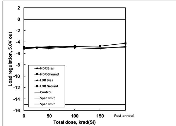
**Figure 33:** ISL75051SEH load regulation, 5.0V out, as a function of biased and grounded high and low dose rate irradiation and subsequent high temperature accelerated post-high dose rate aging at 100°C. The dose rate was 80 rad(Si)/s. Sample size was 6 for the high dose rate cells and 4 for the low dose rate cells, and three control units were used for the high dose rate test. The specification limits are -15.000mV to -0.050mV.
