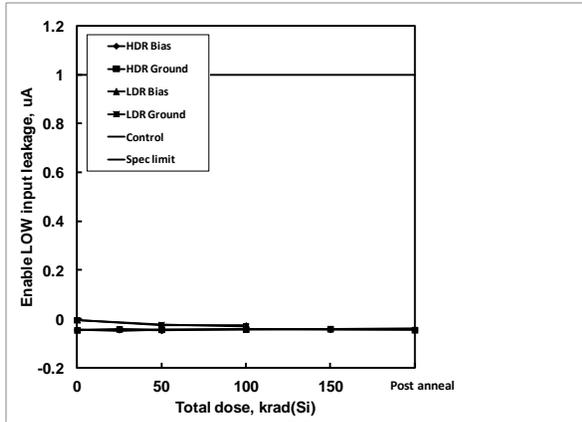
**Figure 2:** ISL75051SEH enable LOW input current as a function of biased and grounded high and low dose rate irradiation and subsequent high temperature accelerated post-high dose rate aging at 100°C. The dose rate was 80 rad(Si)/s. Sample size was 6 for the high dose rate cells and 4 for the low dose rate cells, and three control units were used for the high dose rate test. The specification limits are -0.100µA – +1.000µA.
