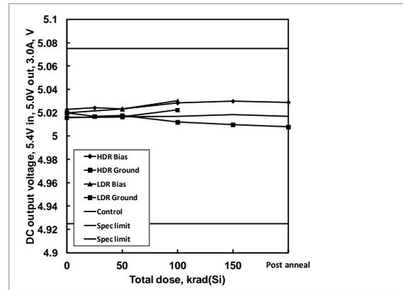
**Figure 25:** ISL75051SEH DC output voltage, 5.0V output, 5.4V input, 3A load, as a function of biased and grounded high and low dose rate irradiation and subsequent high temperature accelerated post-high dose rate aging at 100°C. The dose rate was 80 rad(Si)/s. Sample size was 6 for the high dose rate cells and 4 for the low dose rate cells, and three control units were used for the high dose rate test. The specification limits are 4.9250V – 5.0750V.
