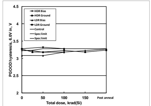
**Figure 45:** ISL75051SEH PGOOD hysteresis, 6.0V in, as a function of biased and grounded high and low dose rate irradiation and subsequent high temperature accelerated post-high dose rate aging at 100°C. The dose rate was 80 rad(Si)/s. Sample size was 6 for the high dose rate cells and 4 for the low dose rate cells, and three control units were used for the high dose rate test. The specification limits are 2.500% to 4.000%.
