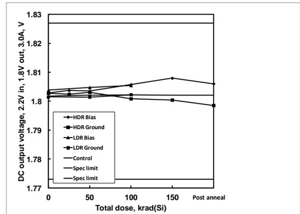
**Figure 21:** ISL75051SEH DC output voltage, 1.8V output, 2.2V input, 3A load, as a function of biased and grounded high and low dose rate irradiation and subsequent high temperature accelerated post-high dose rate aging at 100°C. The dose rate was 80 rad(Si)/s. Sample size was 6 for the high dose rate cells and 4 for the low dose rate cells, and three control units were used for the high dose rate test. The specification limits are 1.7730V – 1.8270V.
