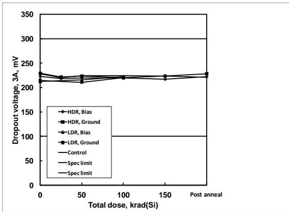
**Figure 51:** ISL75051SEH dropout voltage, 2.5V out, 3A load current, as a function of biased and grounded high and low dose rate irradiation and subsequent high temperature accelerated post-high dose rate aging at 100°C. The dose rate was 80 rad(Si)/s. Sample size was 6 for the high dose rate cells and 4 for the low dose rate cells, and three control units were used for the high dose rate test. The specification limits are 100.000mV to 300.000mV.
