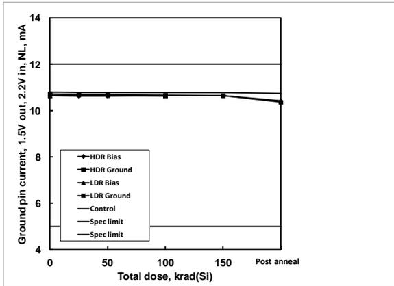
**Figure 35:** ISL75051SEH ground pin current, 1.5V out, 2.2V in, no load, as a function of biased and grounded high and low dose rate irradiation and subsequent high temperature accelerated post-high dose rate aging at 100°C. The dose rate was 80 rad(Si)/s. Sample size was 6 for the high dose rate cells and 4 for the low dose rate cells, and three control units were used for the high dose rate test. The specification limits are 5.000mA to 12.000mA.
