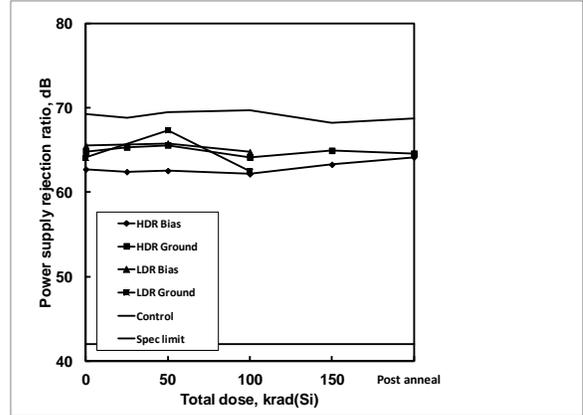
**Figure 52:** ISL75051SEH power supply rejection ratio as a function of biased and grounded high and low dose rate irradiation and subsequent high temperature accelerated post-high dose rate aging at 100°C. The dose rate was 80 rad(Si)/s. Sample size was 6 for the high dose rate cells and 4 for the low dose rate cells, and three control units were used for the high dose rate test. The specification limit is 42dB minimum.
