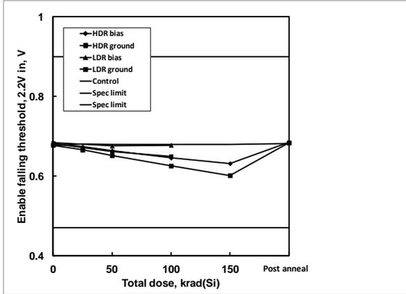
**Figure 6:** ISL75051SEH enable falling threshold, 2.2V input, as a function of biased and grounded high and low dose rate irradiation and subsequent high temperature accelerated post-high dose rate aging at 100°C. The dose rate was 80 rad(Si)/s. Sample size was 6 for the high dose rate cells and 4 for the low dose rate cells, and three control units were used for the high dose rate test. The specification limits are 0.470V – 0.900V.
