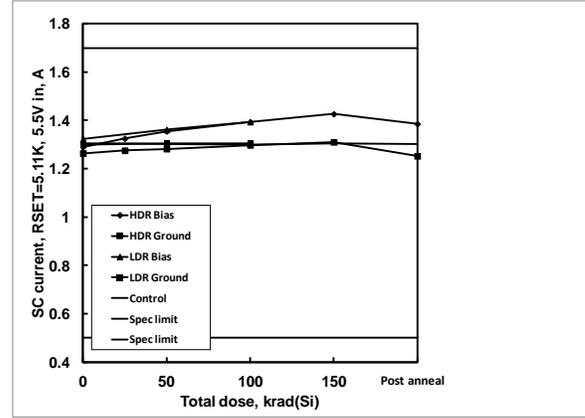
**Figure 55:** ISL75051SEH output short circuit current, RSET=5.11K, 6.0V in, as a function of biased and grounded high and low dose rate irradiation and subsequent high temperature accelerated post-high dose rate aging at 100°C. The dose rate was 80 rad(Si)/s. Sample size was 6 for the high dose rate cells and 4 for the low dose rate cells, and three control units were used for the high dose rate test. The specification limits are 0.500A to 1.700A.
