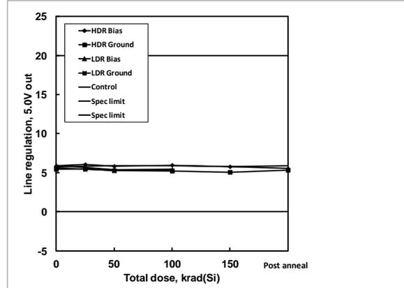
**Figure 32:** ISL75051SEH line regulation, 5.0V out, as a function of biased and grounded high and low dose rate irradiation and subsequent high temperature accelerated post-high dose rate aging at 100°C. The dose rate was 80 rad(Si)/s. Sample size was 6 for the high dose rate cells and 4 for the low dose rate cells, and three control units were used for the high dose rate test. The specification limits are 0mV to +20.000mV.
