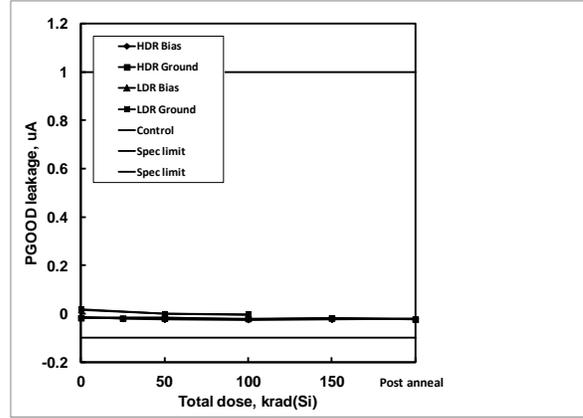
**Figure 40:** ISL75051SEH PGOOD leakage as a function of biased and grounded high and low dose rate irradiation and subsequent high temperature accelerated post-high dose rate aging at 100°C. The dose rate was 80 rad(Si)/s. Sample size was 6 for the high dose rate cells and 4 for the low dose rate cells, and three control units were used for the high dose rate test. The specification limits are -0.010μA to 1.000μA.
