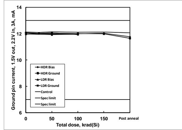
**Figure 36:** ISL75051SEH ground pin current, 1.5V out, 2.2V in, 3A load, as a function of biased and grounded high and low dose rate irradiation and subsequent high temperature accelerated post-high dose rate aging at 100°C. The dose rate was 80 rad(Si)/s. Sample size was 6 for the high dose rate cells and 4 for the low dose rate cells, and three control units were used for the high dose rate test. The specification limits are 7.000mA to 13.000mA.
