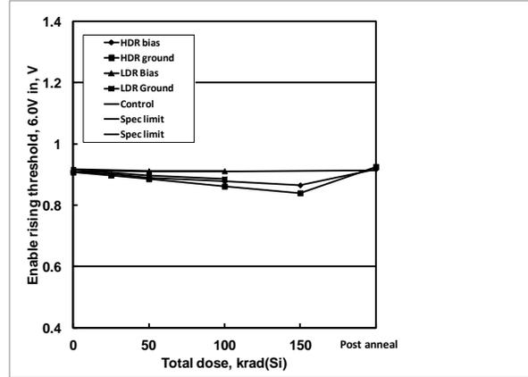
**Figure 8:** ISL75051SEH enable rising threshold, 6.0V input, as a function of biased and grounded high and low dose rate irradiation and subsequent high temperature accelerated post-high dose rate aging at 100°C. The dose rate was 80 rad(Si)/s. Sample size was 6 for the high dose rate cells and 4 for the low dose rate cells, and three control units were used for the high dose rate test. The specification limits are 0.600V – 1.200V.
