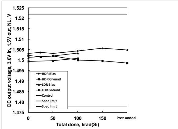
**Figure 18:** ISL75051SEH DC output voltage, 1.5V output, 3.6V input, no load, as a function of biased and grounded high and low dose rate irradiation and subsequent high temperature accelerated post-high dose rate aging at 100°C. The dose rate was 80 rad(Si)/s. Sample size was 6 for the high dose rate cells and 4 for the low dose rate cells, and three control units were used for the high dose rate test. The specification limits are 1.4780V – 1.5220V.
