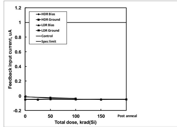
**Figure 4:** ISL75051SEH feedback pin input current as a function of biased and grounded high and low dose rate irradiation and subsequent high temperature accelerated post-high dose rate aging at 100°C. The dose rate was 80 rad(Si)/s. Sample size was 6 for the high dose rate cells and 4 for the low dose rate cells, and three control units were used for the high dose rate test. The specification limits are -1.00µA – +1.00µA.
