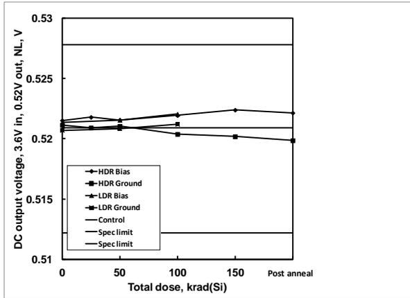
**Figure 14:** ISL75051SEH DC output voltage, 0.52V output, 3.6V input, no load, as a function of biased and grounded high and low dose rate irradiation and subsequent high temperature accelerated post-high dose rate aging at 100°C. The dose rate was 80 rad(Si)/s. Sample size was 6 for the high dose rate cells and 4 for the low dose rate cells, and three control units were used for the high dose rate test. The specification limits are 0.5122V – 0.5278V.
