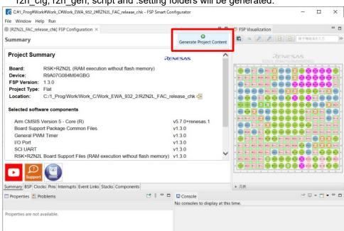
6 In the FSP Configuration pane of the Smart Configurator, click Generate Project Content. The rzn, rzn\_cfg, rzn\_gen, script and .setting folders will be generated.
