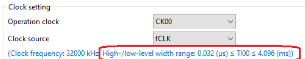
Figure 6-8 High/Low level width min value
