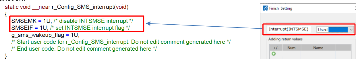
Figure 3-13 r_Config_SMS_interrupt code update
