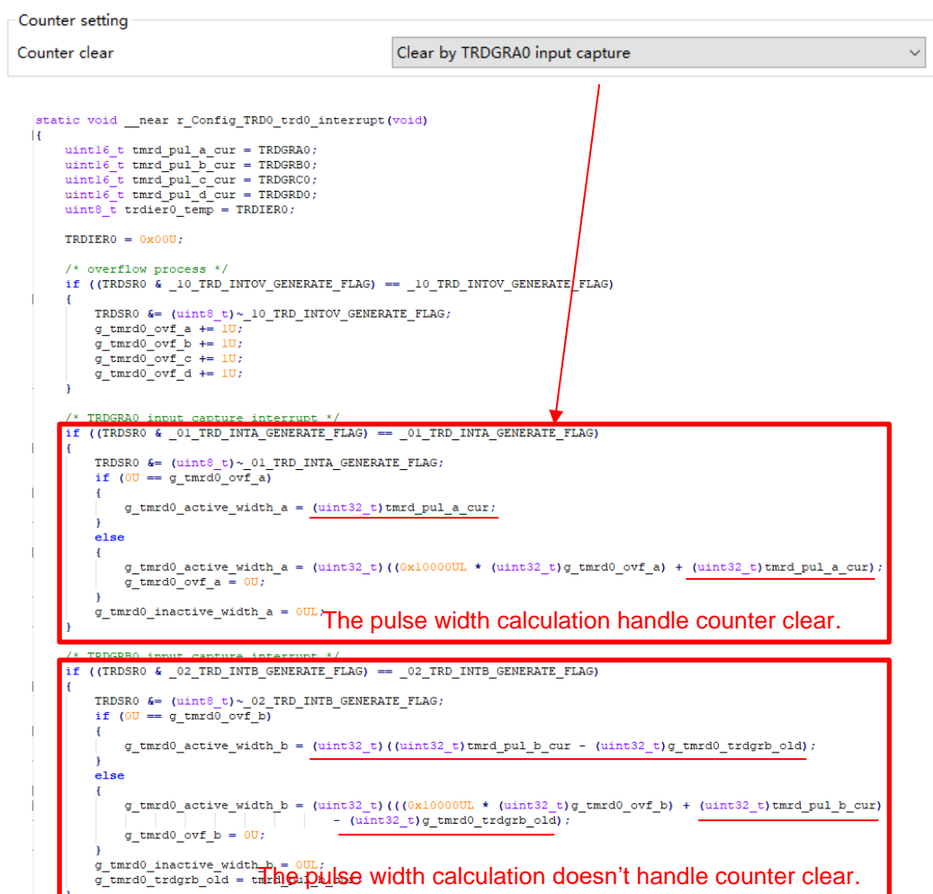
Figure 6-3 Counter clear setting in Input capture function
