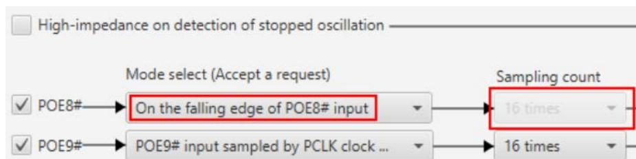
Figure 3-4 Configuration of "Sampling count"
