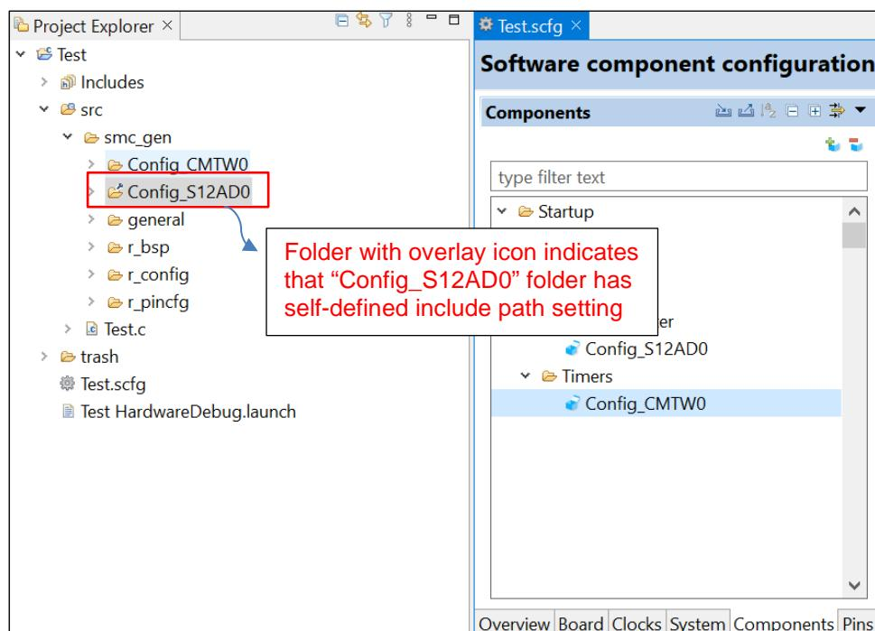
**Figure 6-3 Compare Match Timer component configuration before renaming**
