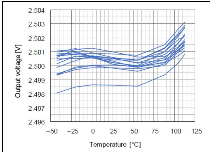
**Figure 39.98** Temperature Dependence of Output Voltage of Voltage Reference (AVCC0 = 5.0 V)
