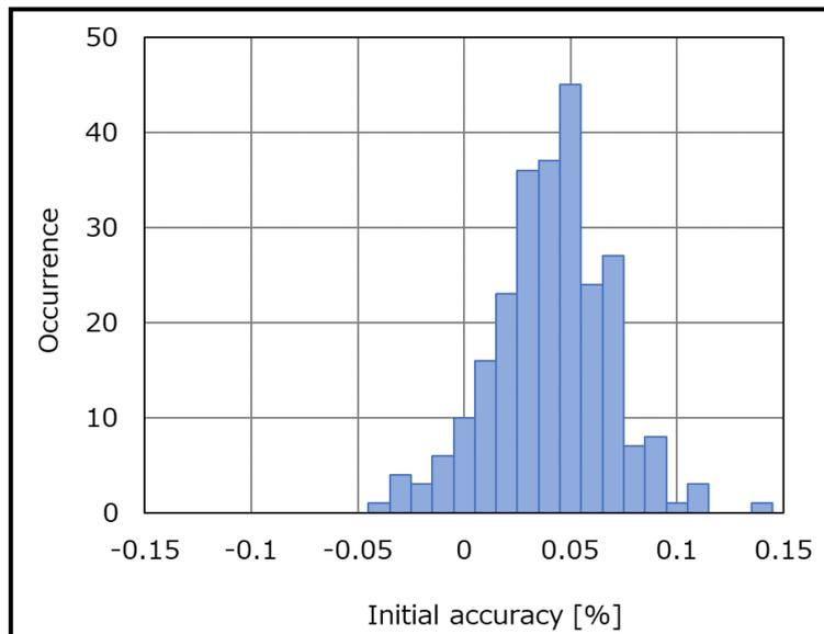
Figure 39.99 Initial Accuracy of Voltage Reference (AVCC0 = 5.0 V)
