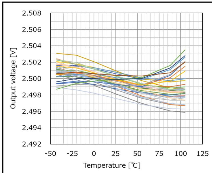
**Figure 39.98** Temperature Dependence of Output Voltage of Voltage Reference (AVCC0 = 5.0 V)
