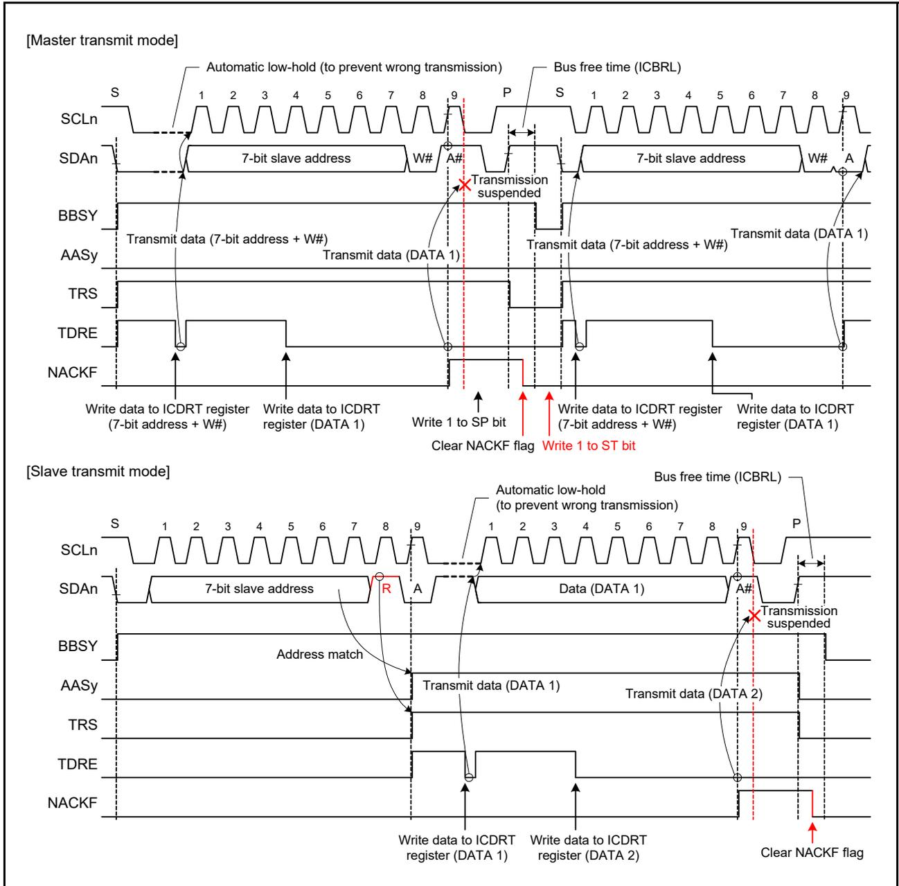
Figure 33.31 Suspension of Data Transmission When NACK is Received (NACK = 1)
