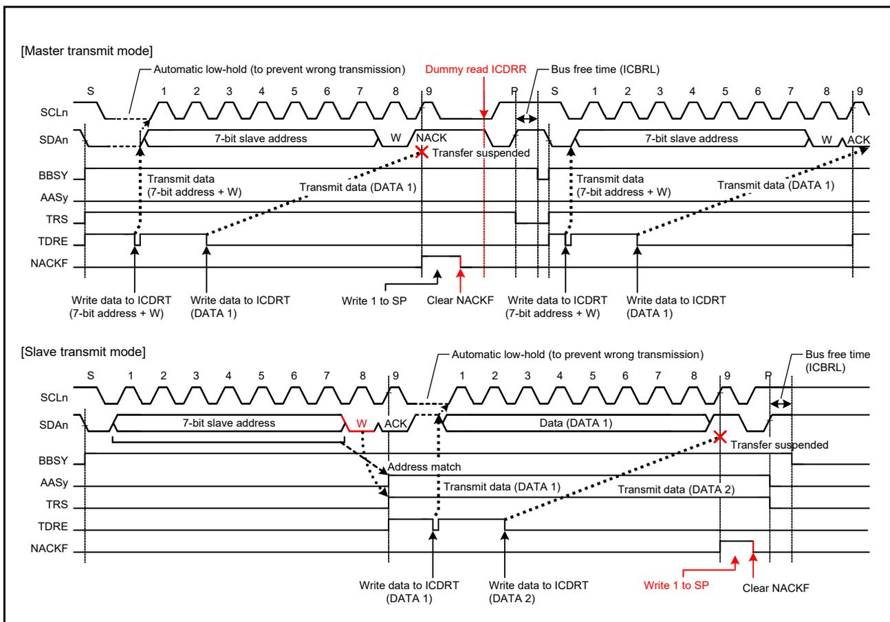
Figure 33.31 Suspension of Data Transfer when NACK is Received (NACKF = 1)
