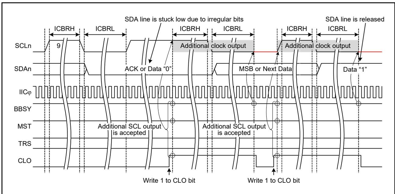
**Figure 33.40 Additional SCL Output Function (CLO Bit)**
