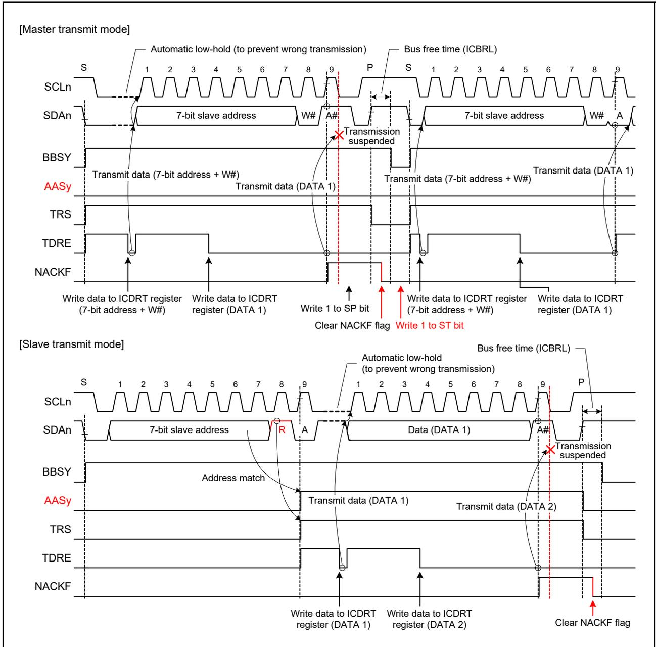
Figure 22.30 Suspension of Data Transmission When NACK is Received (NACK = 1)
