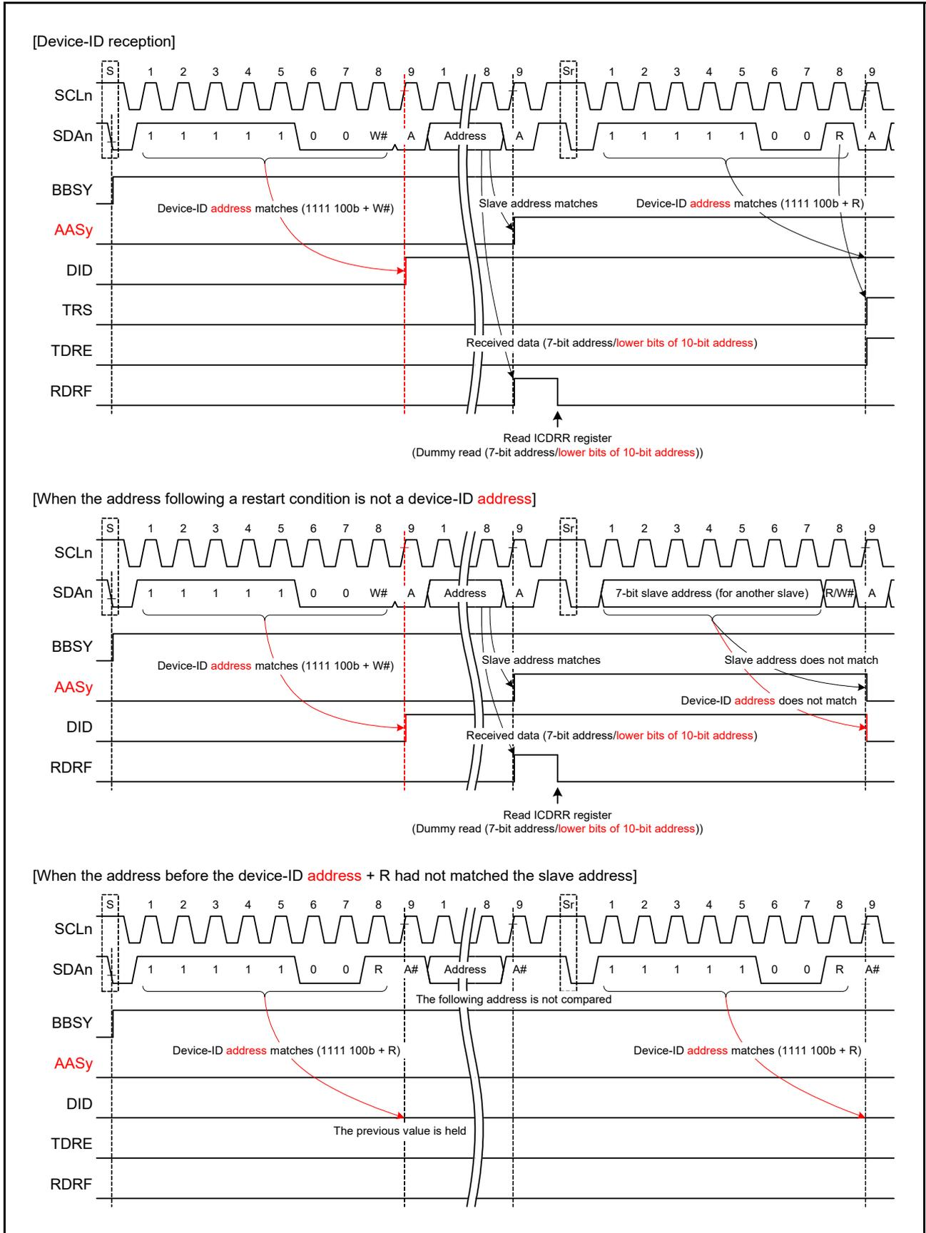
Figure 22.27 Set/Clear Timing of the AASY and DID Flags during Reception of Device-ID Address
