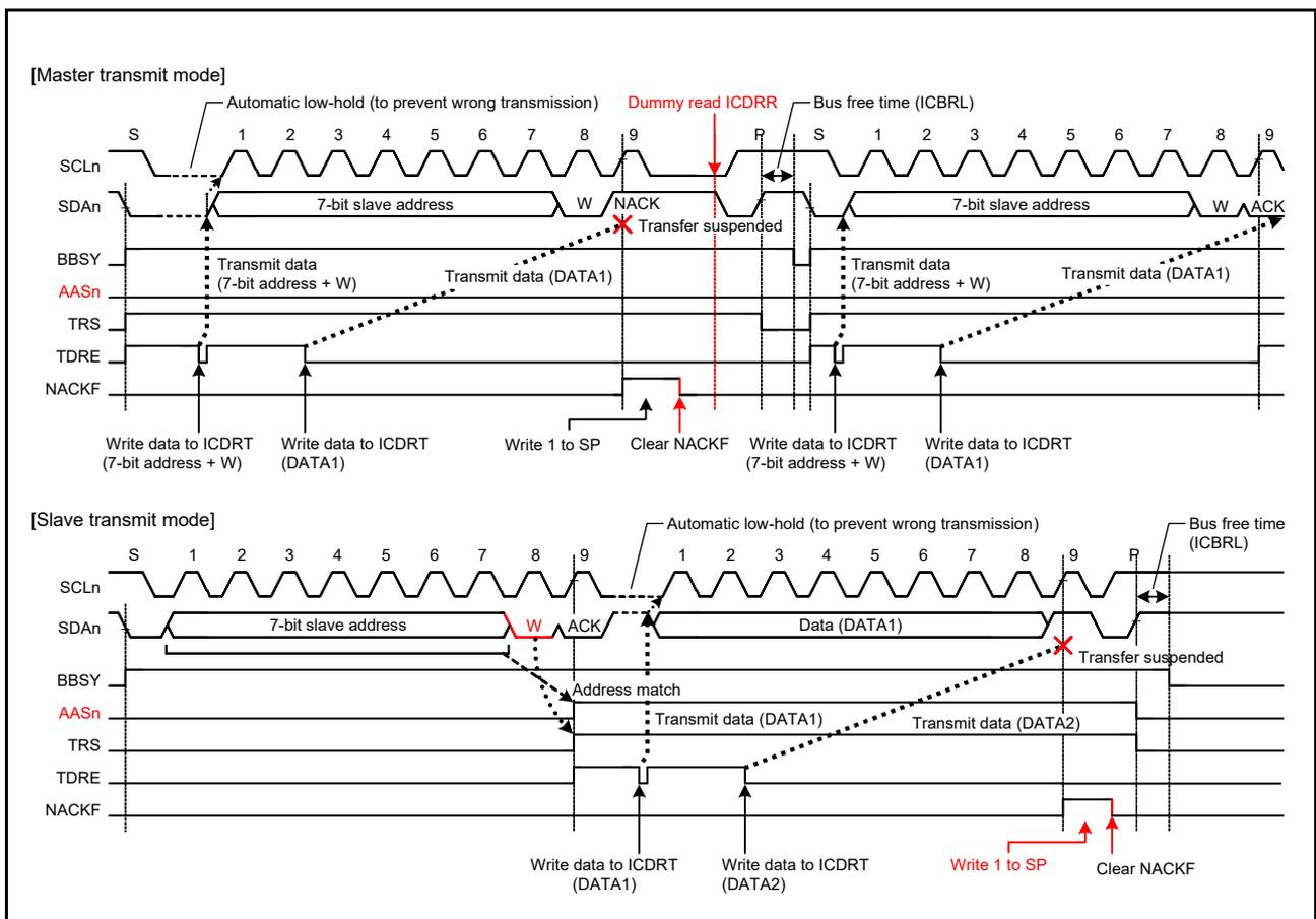
Figure 22.30 Suspension of Data Transfer when NACK is Received (NACKF = 1)
