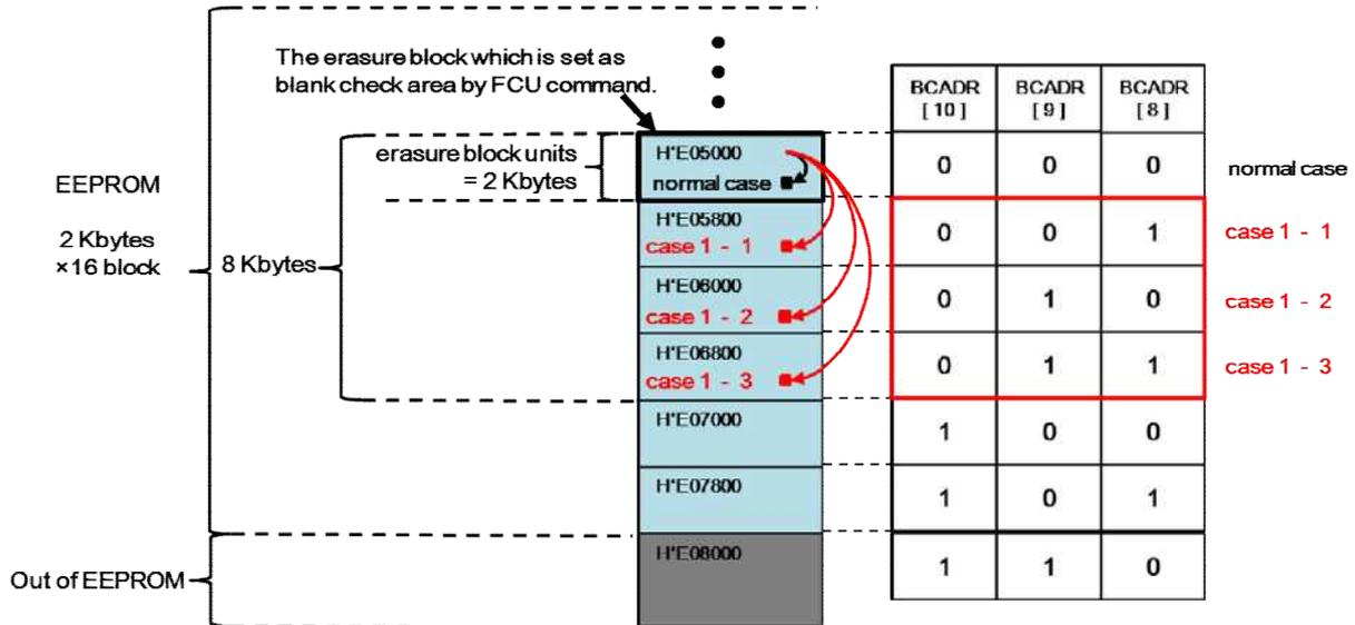
Figure 2 . Example of malfunction ( Case1 )
