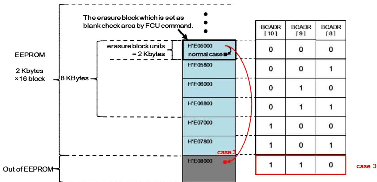
Figure 4 . Example of malfunction ( Case 3 )
