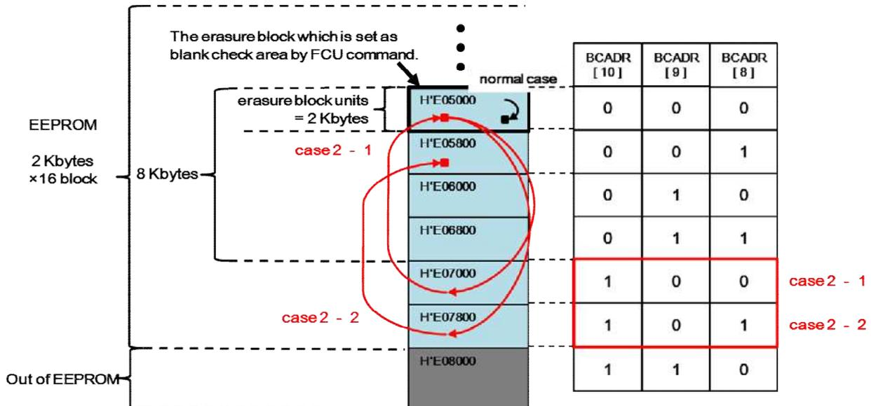
Figure 3 . Example of malfunction ( Case 2 )
