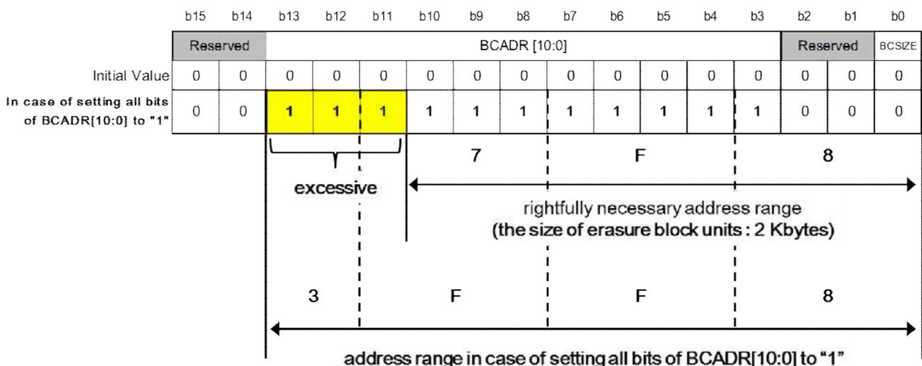
Figure1 . Address range in case of setting all bits of BCADR[10:0] to "1" and the rightfully necessary address range.
