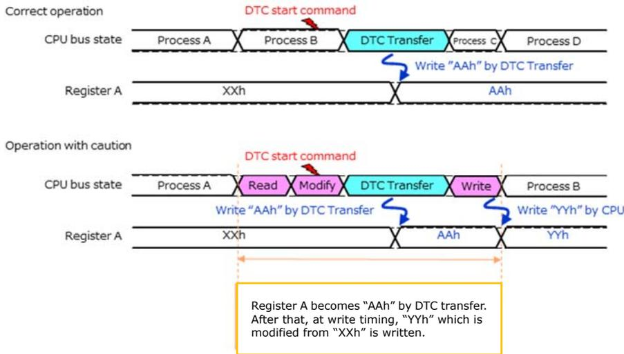
Figure 3. Condition of CPU bus and specific register
