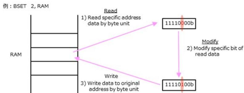
Figure 4. operation of Read-Modify-Write instruction
