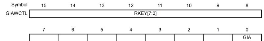
The RKEY[7:0] bits contain the key code to control rewriting of the GIAWCTL register. When rewriting the GIA bit, set RKEY[7:0] to **A4H** and then write to all 16 bits of this register at once. The RKEY[7:0] bits return 00H when read.
