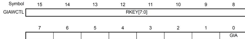
The RKEY[7:0] bits contain the key code to control rewriting of the GIAWCTL register. When rewriting the GIA bit, set RKEY[7:0] to **C4H** and then write to all 16 bits of this register at once. The RKEY[7:0] bits return 00H when read.
