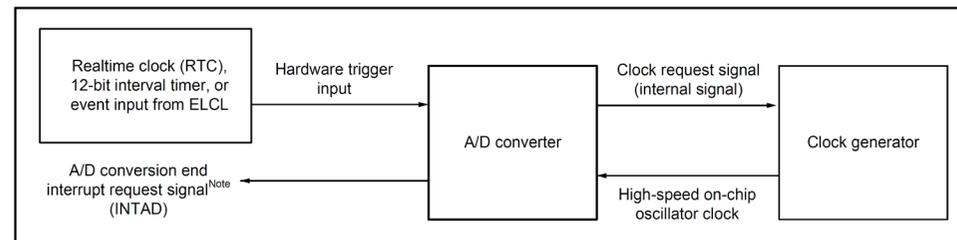
When using the SNOOZE mode function, the initial setting of each register is specified before switching to the STOP mode (for details about these settings, see **Figure 12 - 45 Flowchart for Setting up SNOOZE Mode (Hardware Trigger)**). Just before moving to STOP mode, set bit 2 (AWC) of A/D converter mode register 2 (ADM2) to 1. After the initial settings are specified, set bit 0 (ADCE) of A/D converter mode register 0 (ADM0) to 1.
