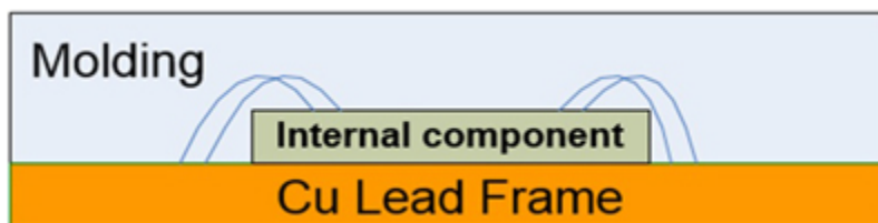
Figure 4. ISL8203M internal structure
