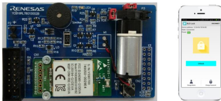
Figure 6. The smart lock system
