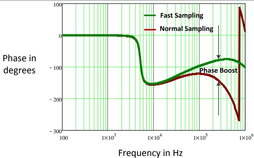
**Figure 4 – Phase boost at high frequencies**
