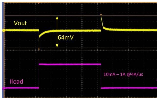
Figure 5. ISL80510 transient response (2.2V<sub>in</sub>, 1.8V<sub>out</sub>)
